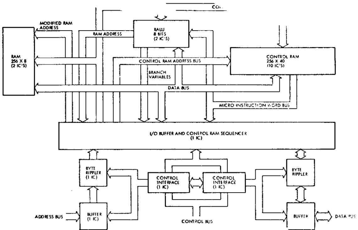
**Figure 2 CORE PROCESSOR**
