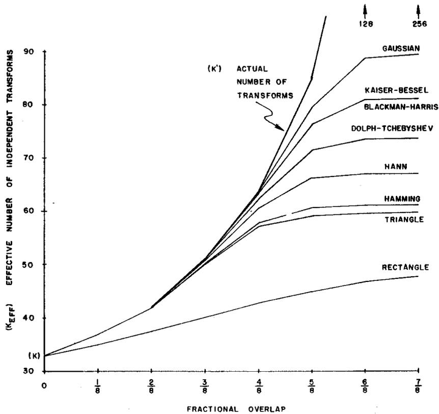
**FIGURE 6. EQUIVALENT NUMBER OF INDEPENDENT TRANSFORMS AS A FUNCTION OF FRACTIONAL OVERLAP FOR VARIOUS CLASSIC WINDOWS**
