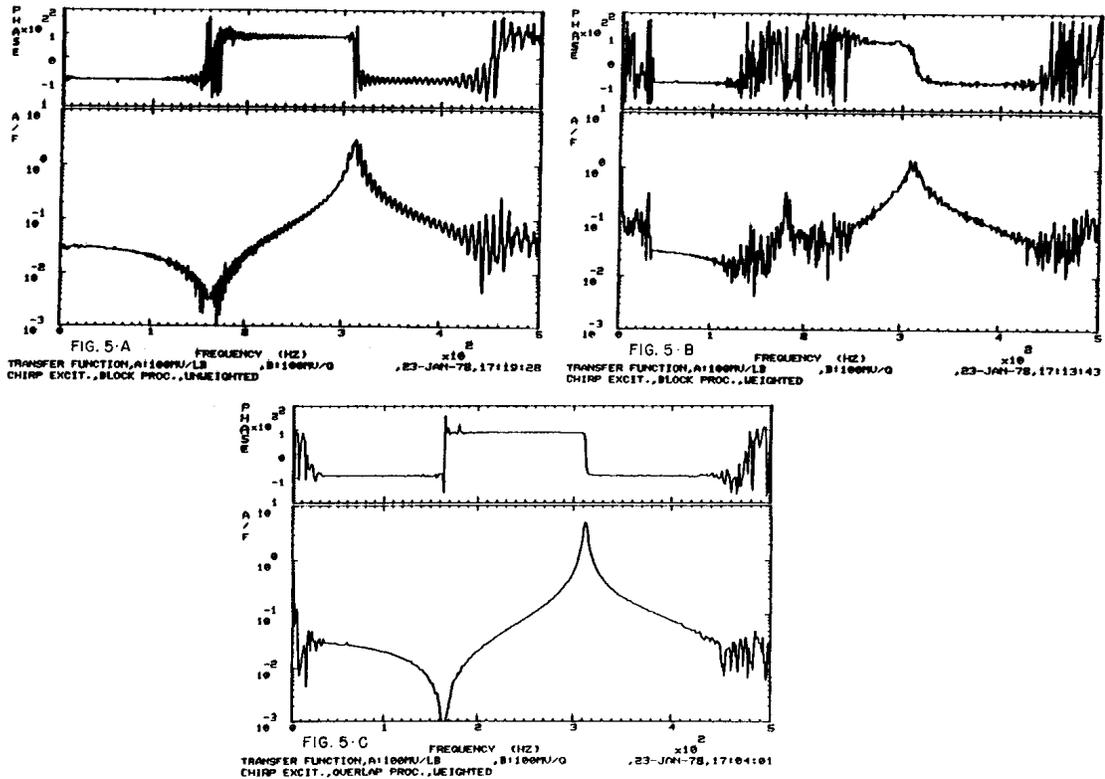
**FIGURE 5. SWEEP FREQUENCY TRANSFER FUNCTION WITH VARIOUS COMBINATIONS OF OVERLAP AND WINDOWING**
