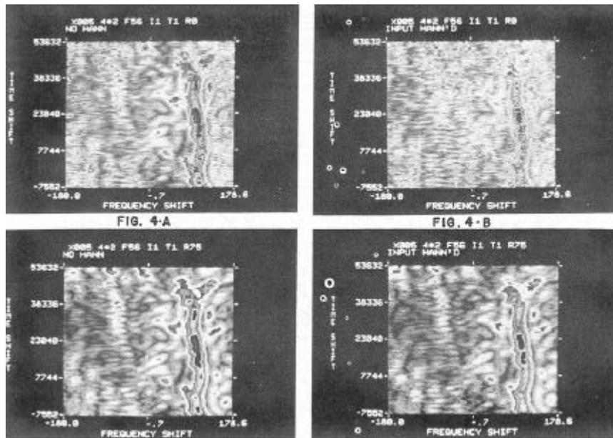
**FIGURE 4. NORMALIZED (TIME-DOPPLER) AMBIGUITY SURFACE WITH VARIOUS COMBINATIONS OF OVERLAP AND WINDOWING**
