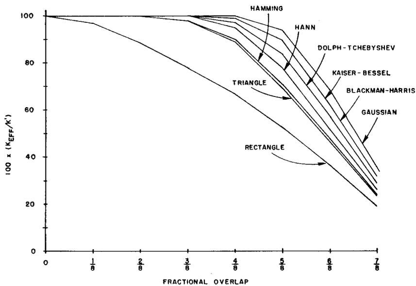
**FIGURE 7. RATIO ( $K_{\text{EFF}}/K'$ ) AS A FUNCTION OF FRACTIONAL OVERLAP FOR VARIOUS CLASSIC WINDOWS**
