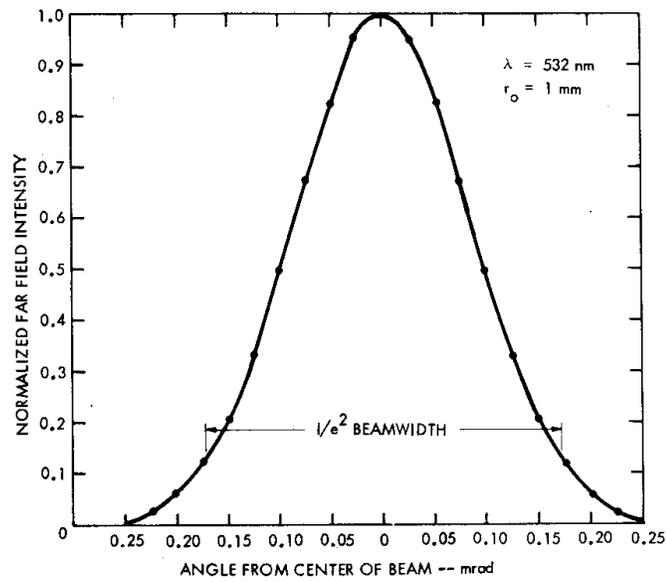
Figure 1. Gaussian For Field Angular Distribution
