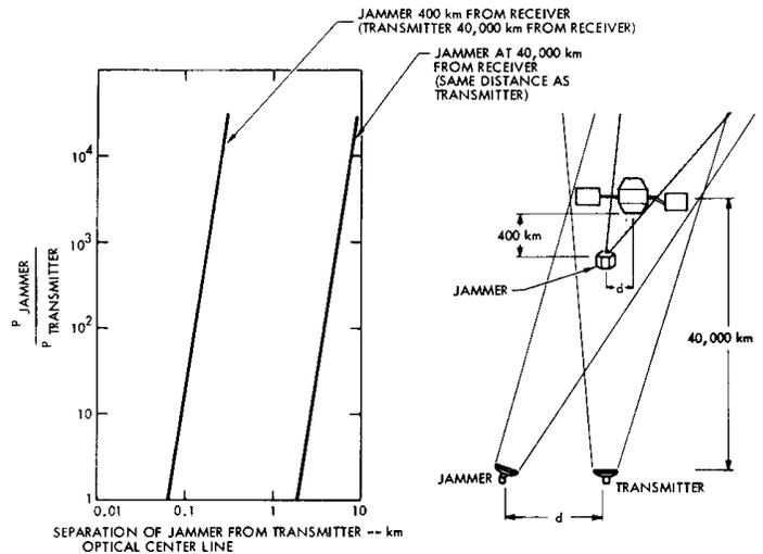
**Figure 10. Optical Receiver Jamming Considerations**
