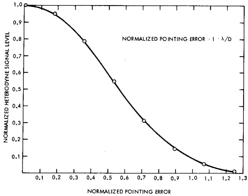
**Figure 8. Heterodyne Signal Drop As A Function Of Receiver Pointing Error**
