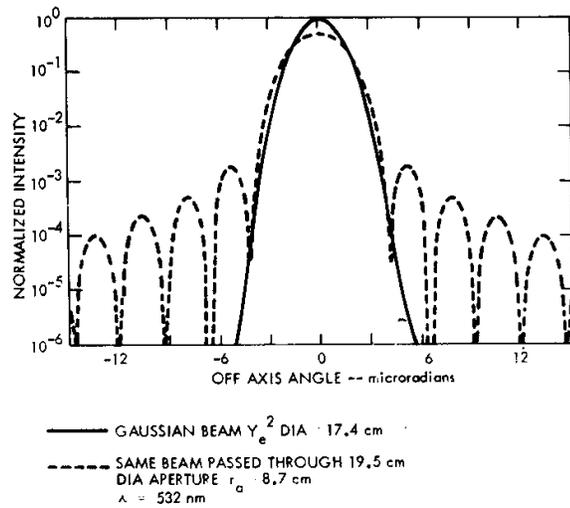
Figure 2. Far-field Intensity Distribution For Circular Aperture Normalized To An Infinite Aperture
