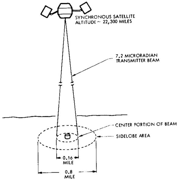
**Figure 9. Optical Transmitter Security Considerations**
