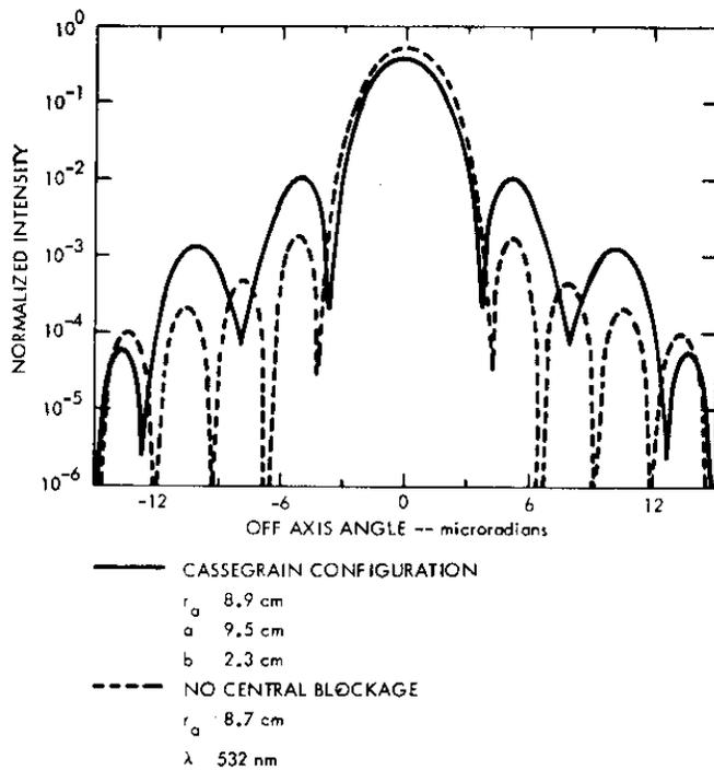
**Figure 5. Far-field Intensity Distribution For Cassegrain Normalized To An Infinite Aperture With Zero Secondary Blockage**
