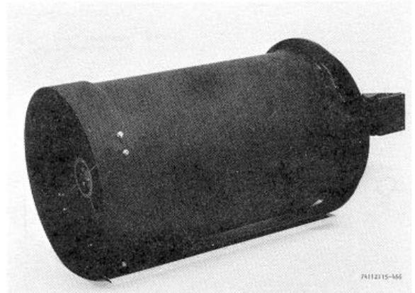
**Figure 6. Beryllium Transmitter Antenna**
