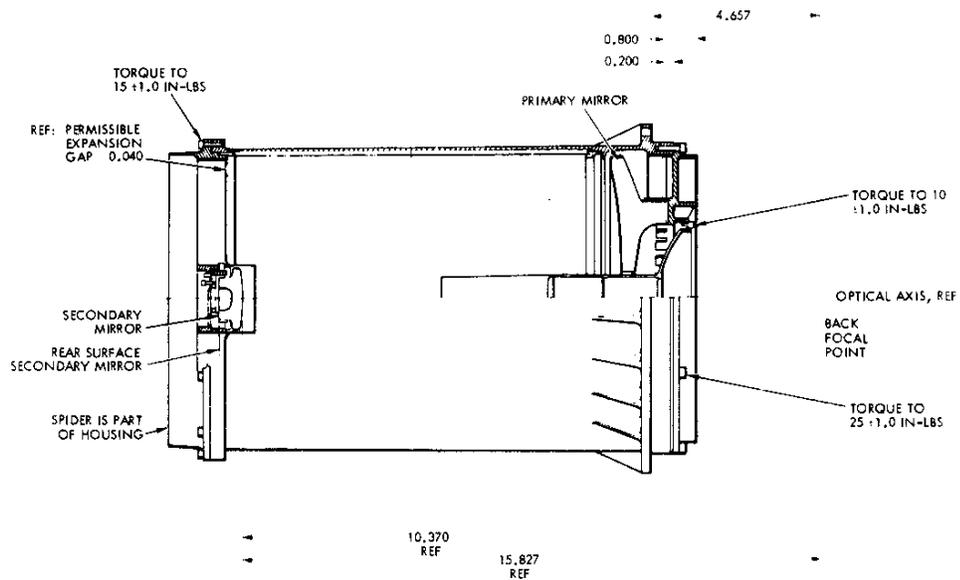
**Figure 7. Invar/Cervit Transmitter Antenna**
