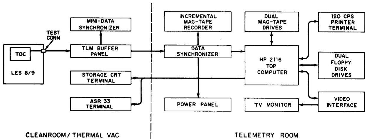
**Fig. 7. Integration and Test Configuration**
