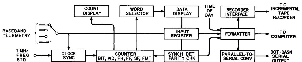
Fig. 2. Data Synchronizer Block Diagram
