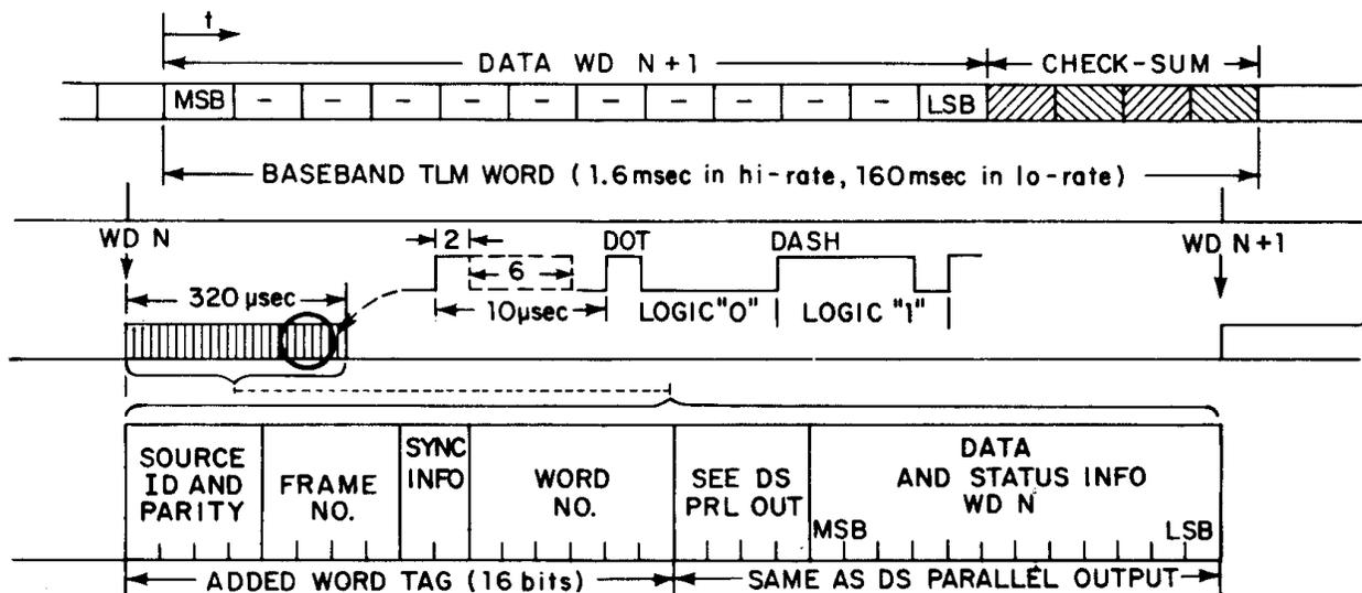
**Fig. 4. Data Synchronizer Serial Output**
