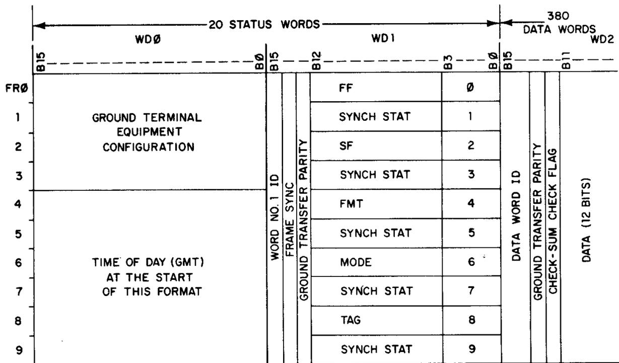
**Fig. 3. Data Synchronizer Parallel Output**
