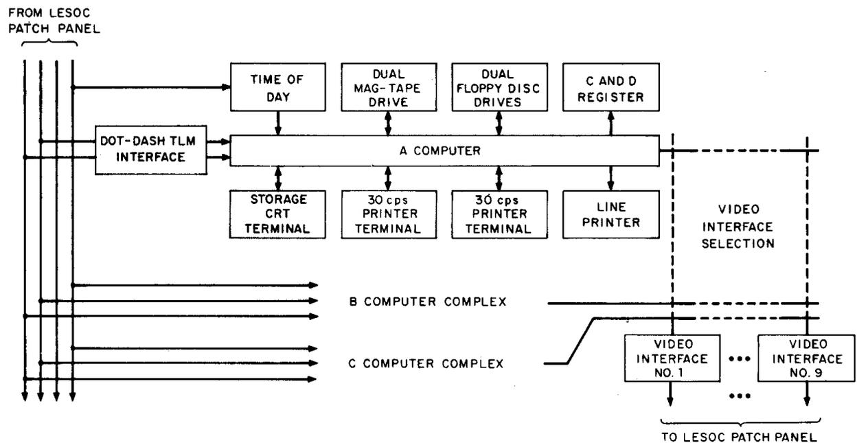
Fig. 5. Telemetry Computer System
