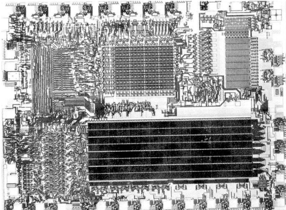
**Fig. 2:** The INTEL 8022 Microcomputer consists of an A to D converter 2K bytes of ROM, 64 bytes of RAM, 8 bit CPU, clock and oscillator and 26 digital I/O lines. Die size is 200 x 225 mils. (Photo courtesy Intel Corporation)
