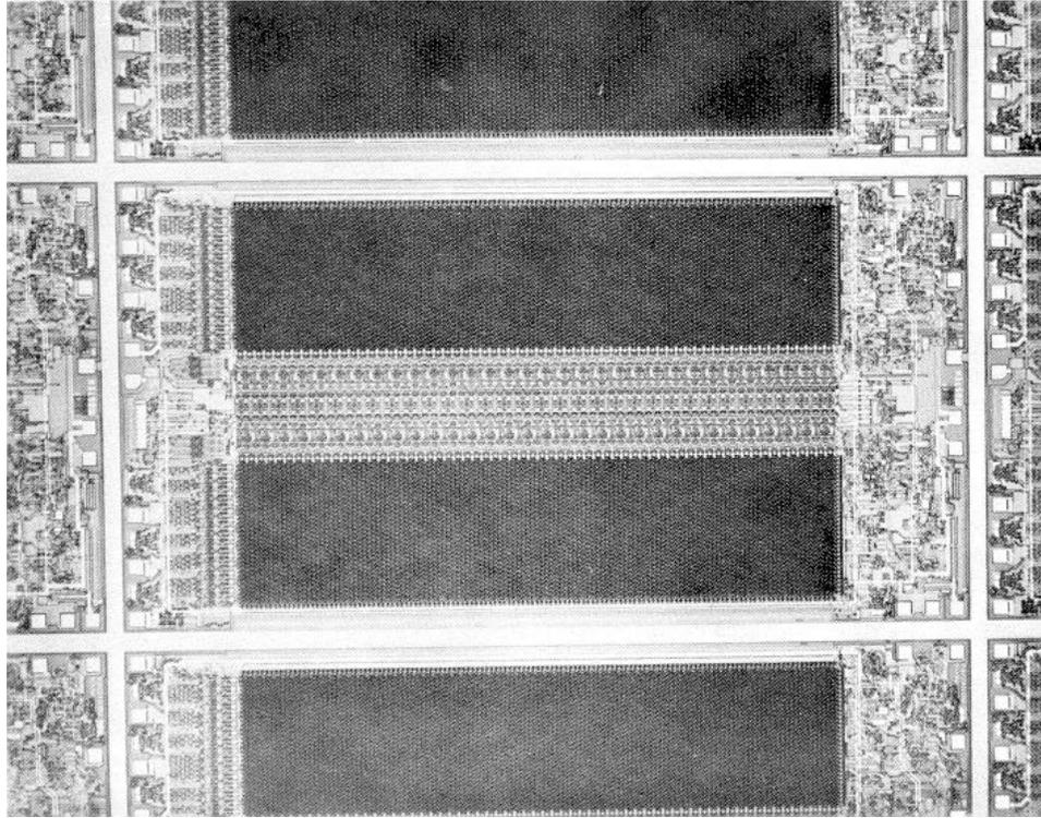
**Fig. 4:** The MK4116 (P)-2 is a 16,384 x 1 bit dynamic RAM on a 105 x 205 mil die. It has a cycle time of 320 nanoseconds and consumes 462 mw. (Photo courtesy MOSTEK Corporation)
