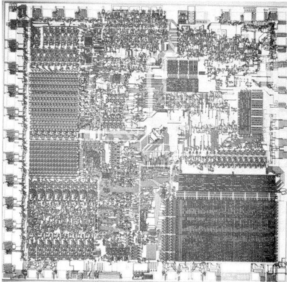
**Fig.3:** The INTEL 8086, 16 bit NMOS microprocessor on a 225 x 225 mil silicon die contains 29,000 transistors. It executes over 200 instructions, including multiply and divide. (Photo courtesy Intel Corporation)
