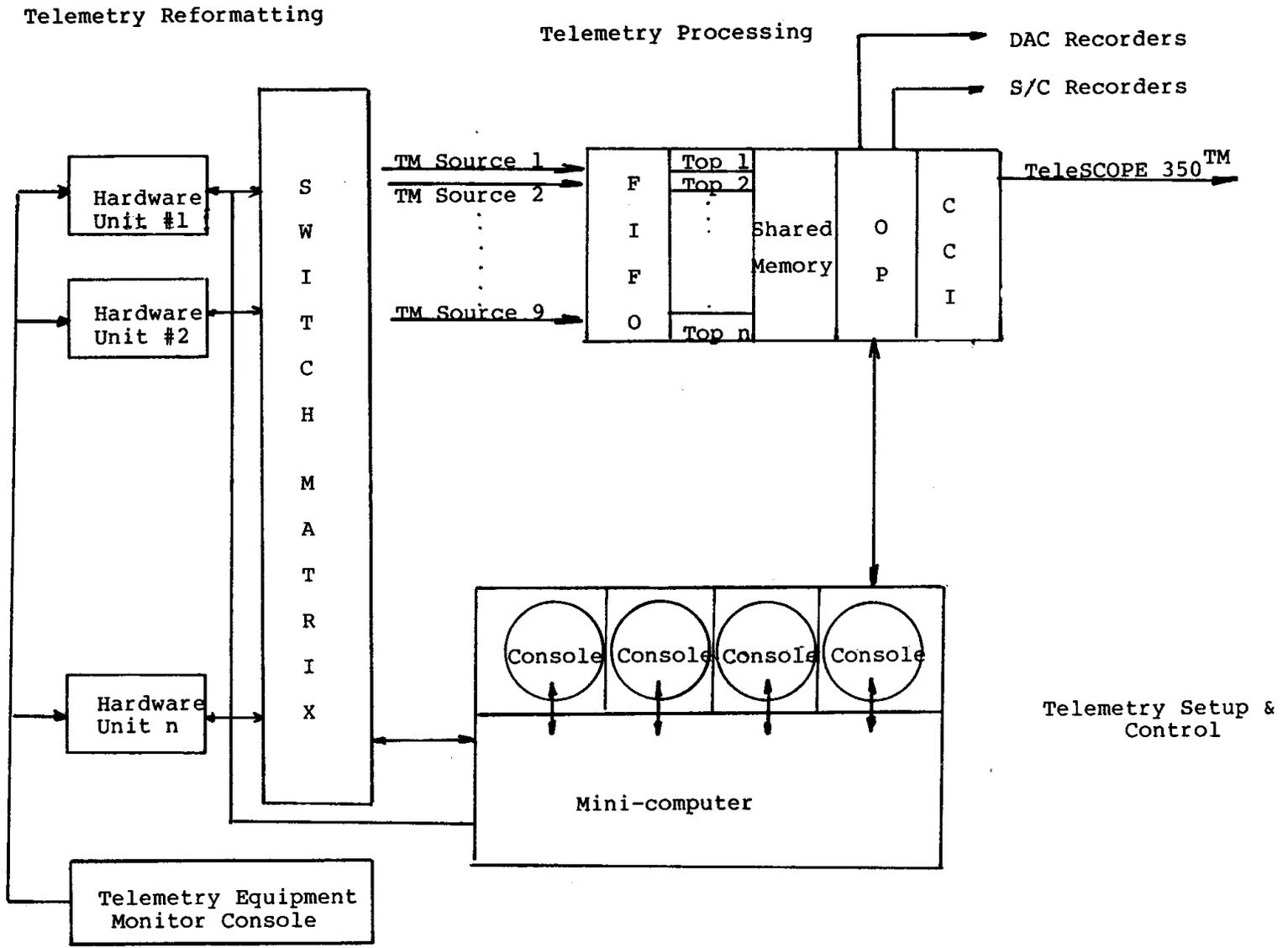
Figure 1 - Telemetry Handling Subsystem
