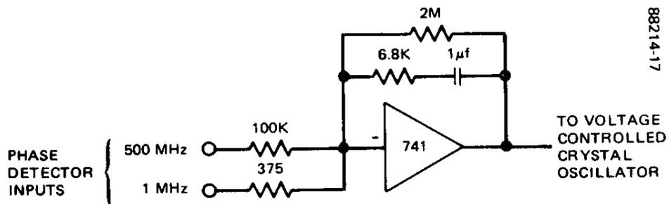
Figure 5 - Acquisition Test Loop Filter
