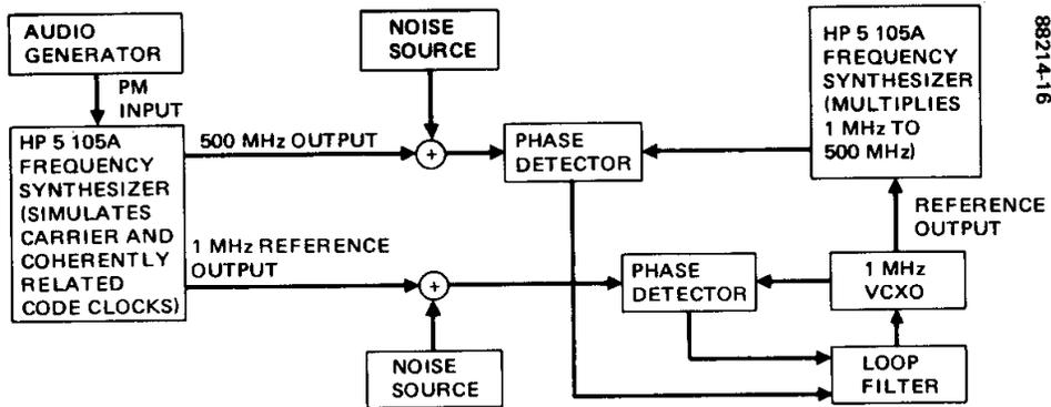
Figure 4 - Acquisition Test Block Diagram
