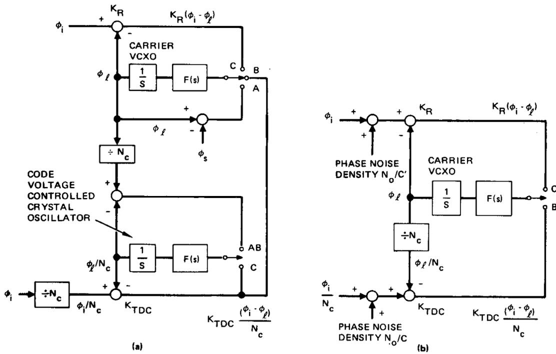
Figure 2 - Frequency Control Circuitry Phase Propagation
