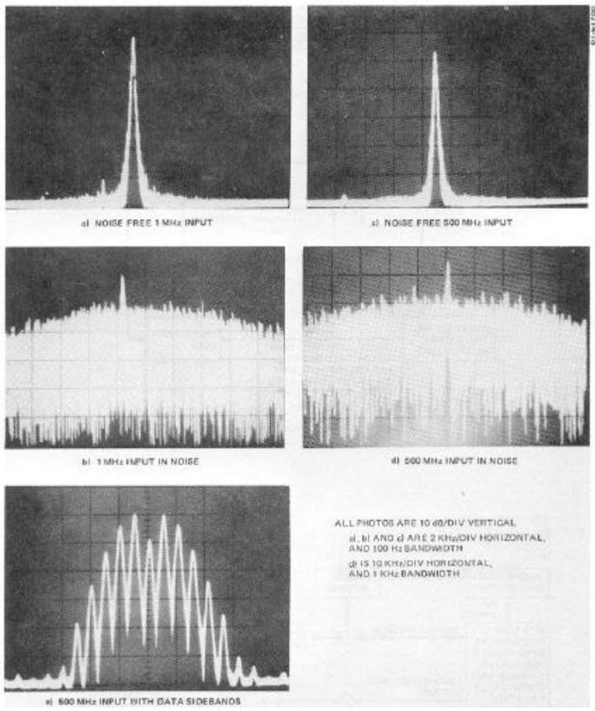
**Figure 6 - Analyzer Photographs of Incoming Signals**
