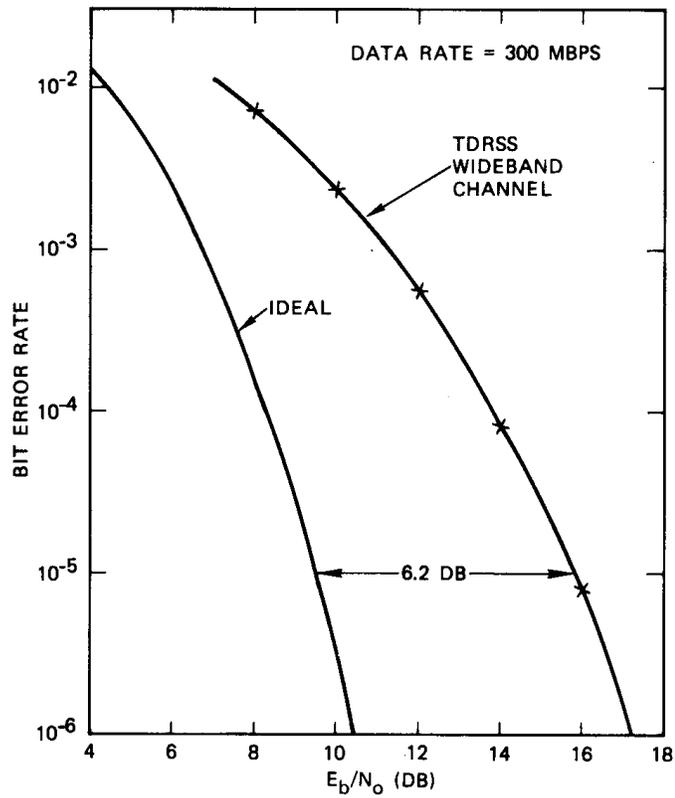
Figure 5. Bit Error Rate Versus  $E_b/N_0$  : TDRSS Wideband Channel
