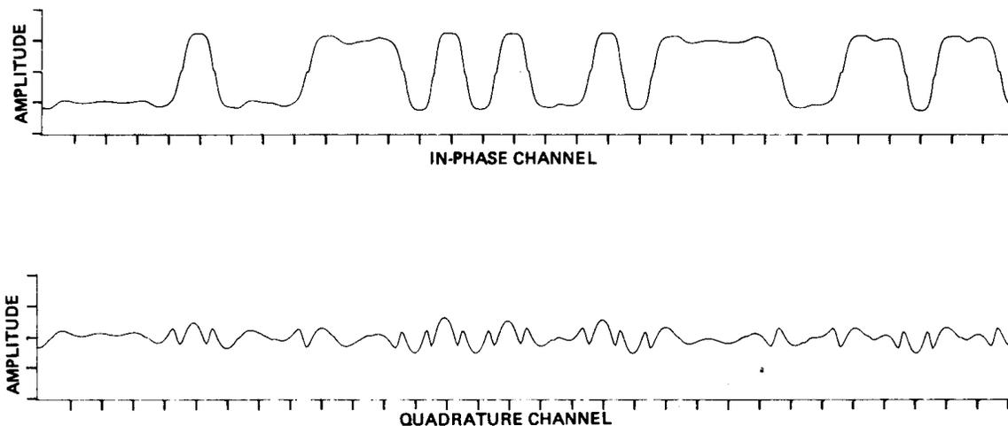
Figure 6. Generated Crosstalk at Output of Spacecraft TWTA - Static Q-Channel
