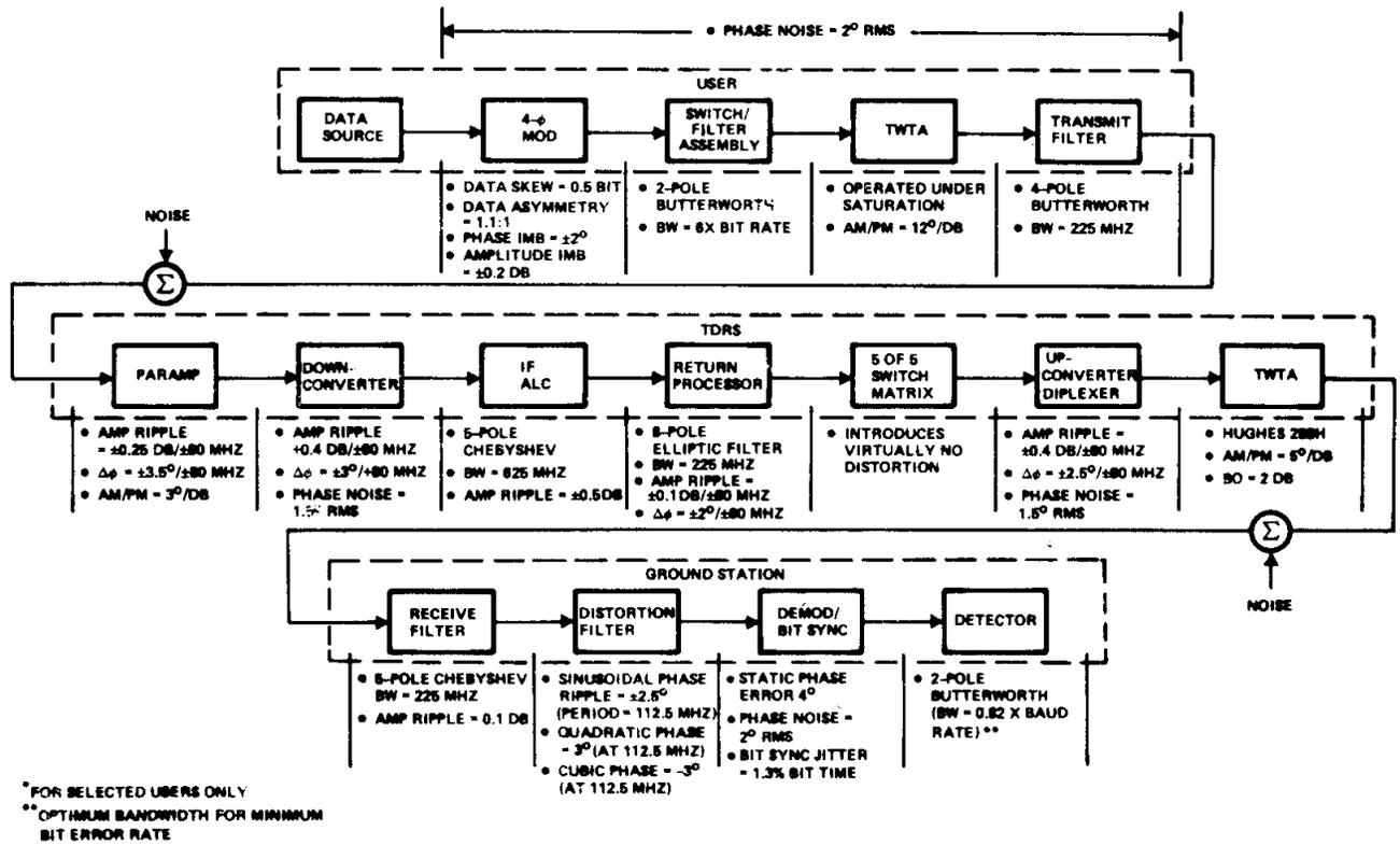
Figure 2. TDRSS Wideband Data Channel: Block Diagram
