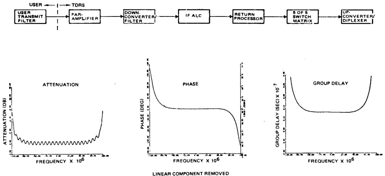
Figure 3. Wideband Channel Frequency Response (Prior to Spacecraft TWTA)
