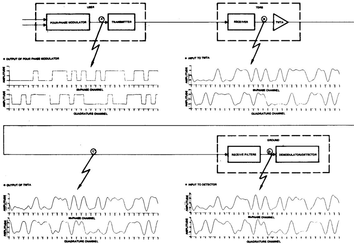
Figure 4. Channel Waveforms
