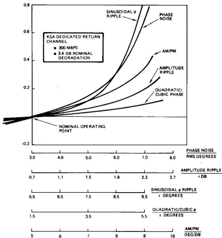
Figure 7. Transponder Parameter Sensitivity Analysis
