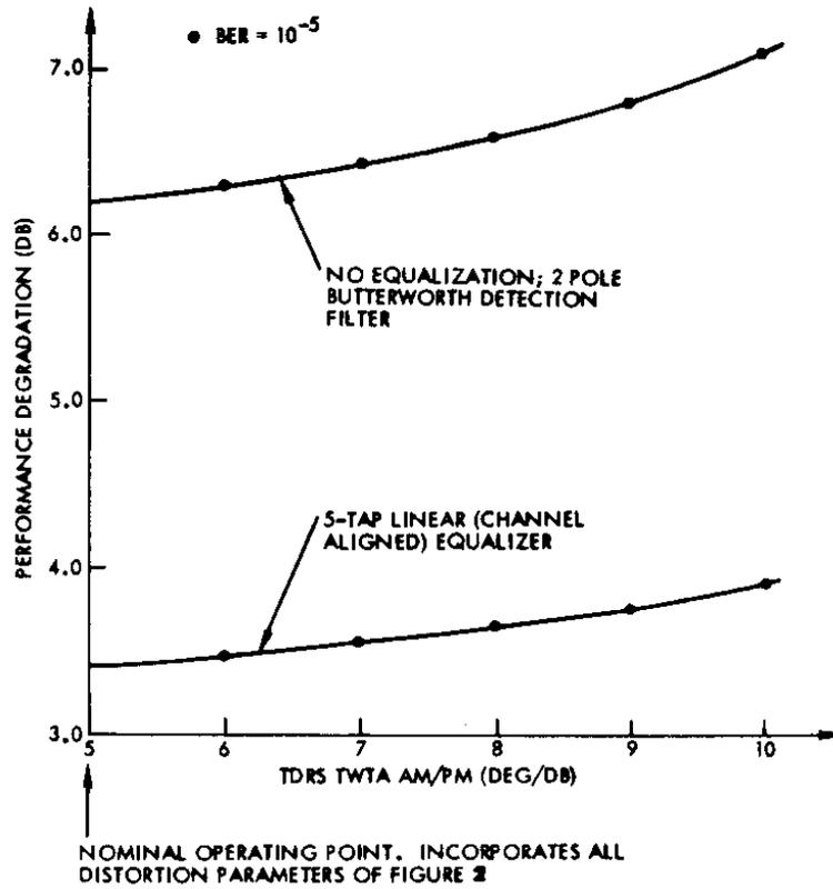
**Figure 9. Effect of Adaptive Equalization on AM/PM-Induced Performance Degradation**
