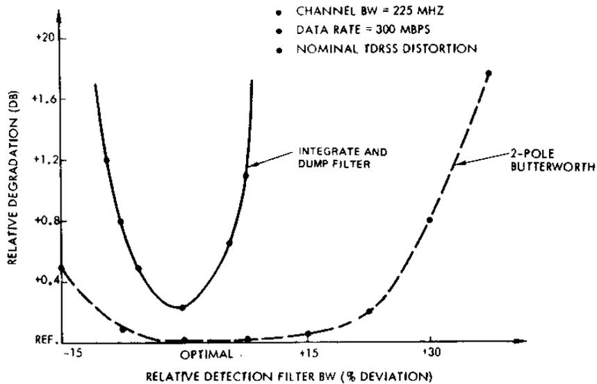
**Figure 10. Performance Comparison: 2-Pole Butterworth Versus Integrate and Dump Detection**
