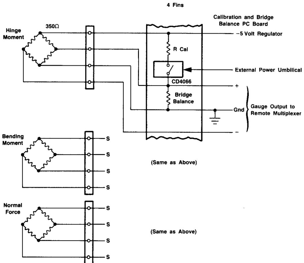
Figure 5. ASALM Strain Gauge Measurement System
