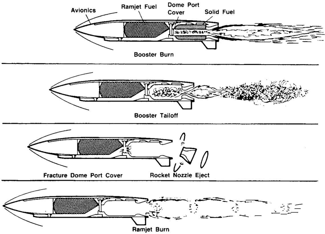
**Figure 1. The Advanced Strategic Air Launched Missile (ASALM) Rocket/Ramjet Concept**
