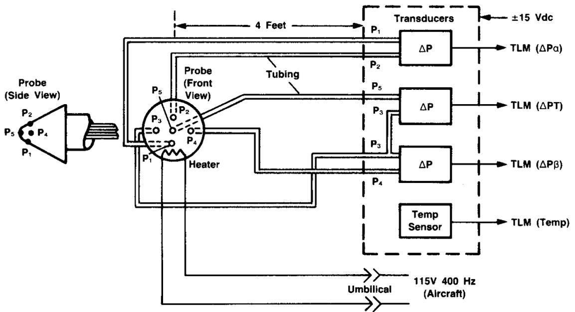
Figure 4. The ASALM Air Data Measurement Probe System
