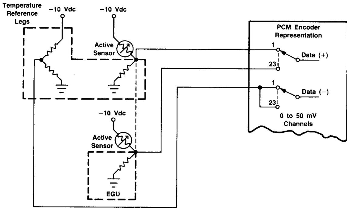
**Figure 2. ASALM Temperature Measuring System, Showing Connections to the Pulse Code Modulator (PCM) Encoder.**
