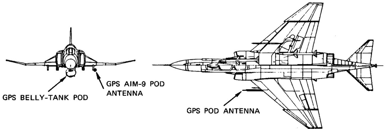
**Figure 1 - F-4 Aircraft with GPS Equipment Locations**
