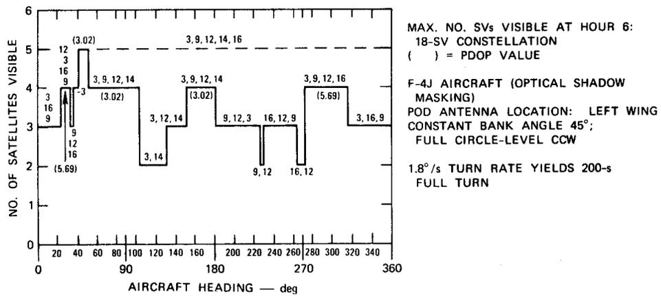
**Figure 8 - Number of Satellites Visible in Counterclockwise Full Circle at 45° Constant Bank Angle**
