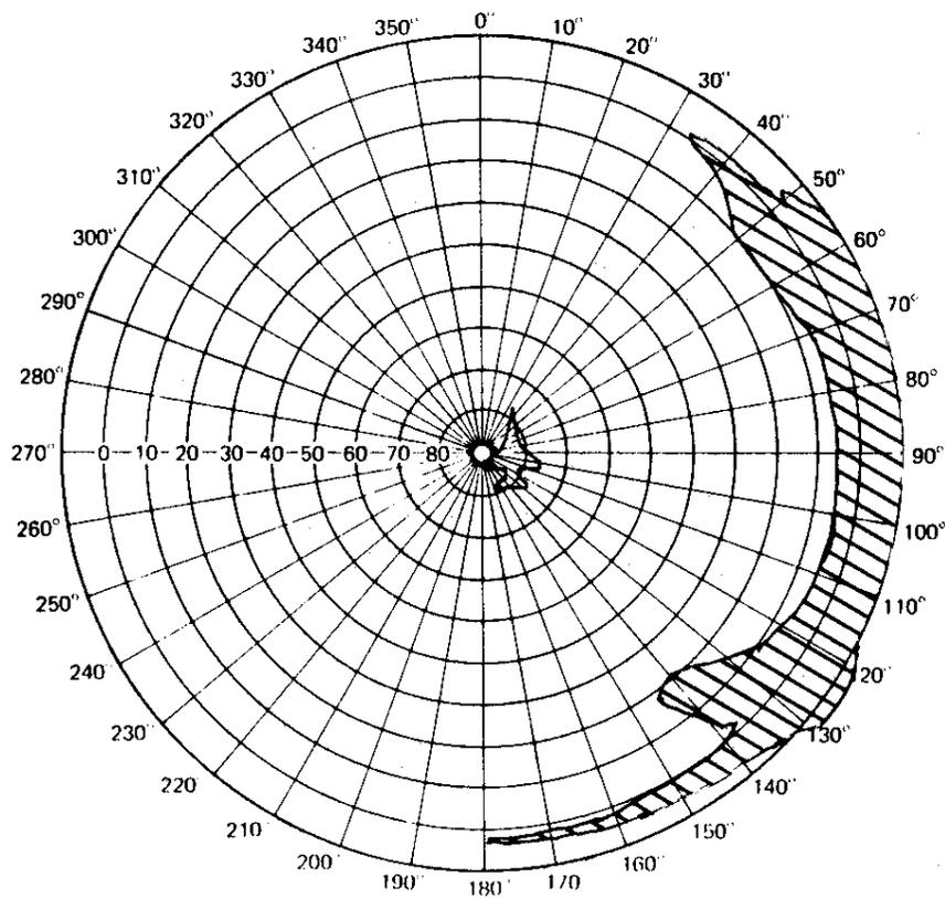
**Figure 9a - Shadowgram for F-16 Aircraft with Wing-Tip-Mounted GPS Antenna Pod**
