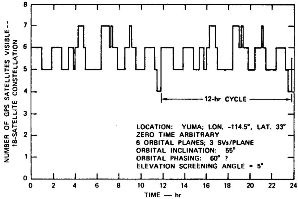
**Figure 4 - Number of GPS Satellites Visible at Yuma in an 18-Satellite Constellation of the Type Planned**
