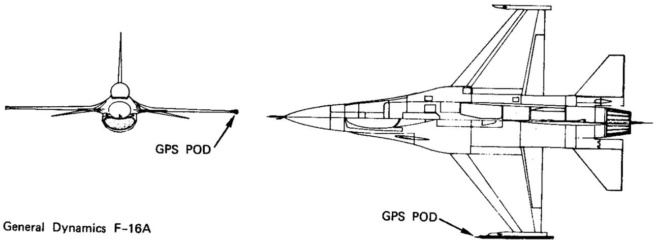
**Figure 3a - F-16 Aircraft with Typical GPS Pod Location**
