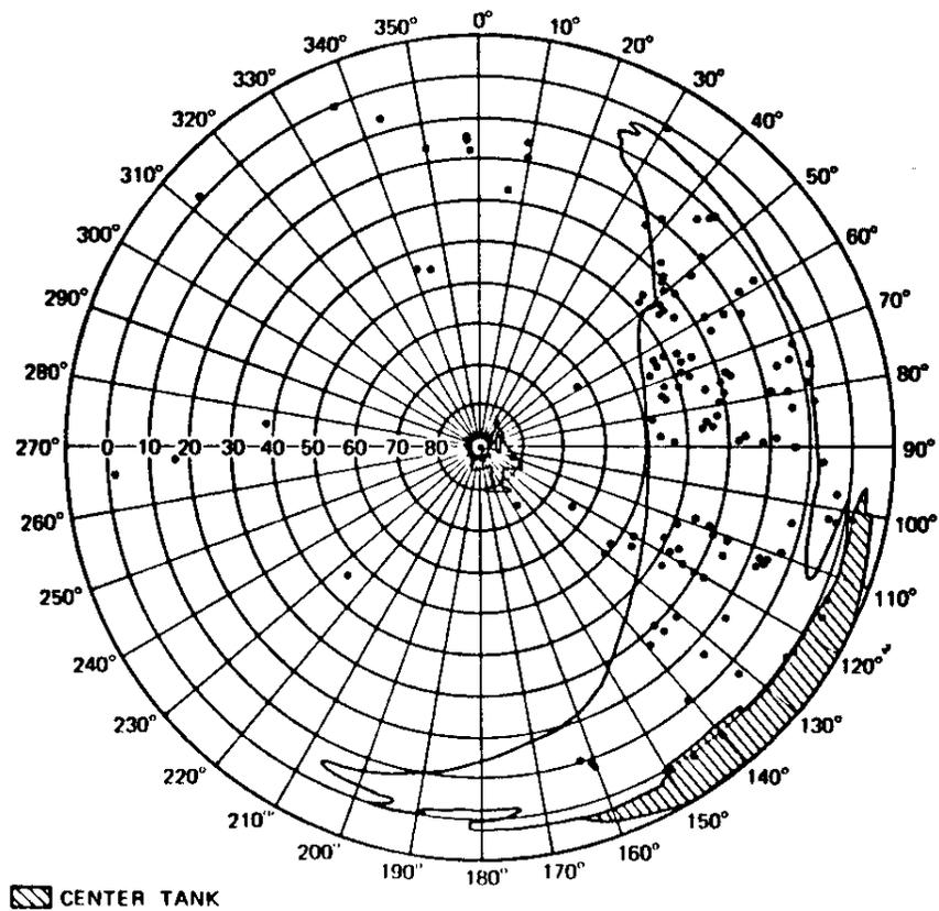
**Figure 2 - Loss-of-Lock in Relation to F4-J Aircraft Optical Shadow From AIM-9 Pod Mounted GPS Antenna (Mission 4075)**
