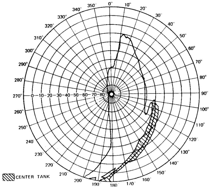
**Figure 7 - Optical Shadow of F4-J Aircraft at 45° Bank Angle (left) From Pod Antenna on Left Wing**
