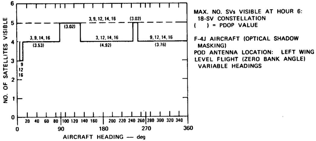
**Figure 6 - Number of Satellites Visible in Level Flight (F4-J with pod antenna)**
