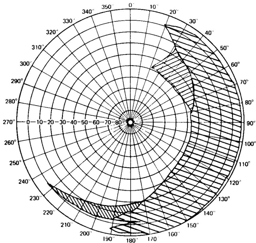
**Figure 9b - Shadowgram for F-14 Aircraft with GPS Pod Antenna Mounted as in Figure 3**
