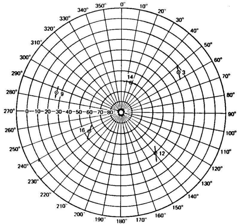
**Figure 5 - Azimuth and Elevation of Satellites at 0600 hrs ( $\pm 15$  min; best four-satellite PDOP = 3.02)**
