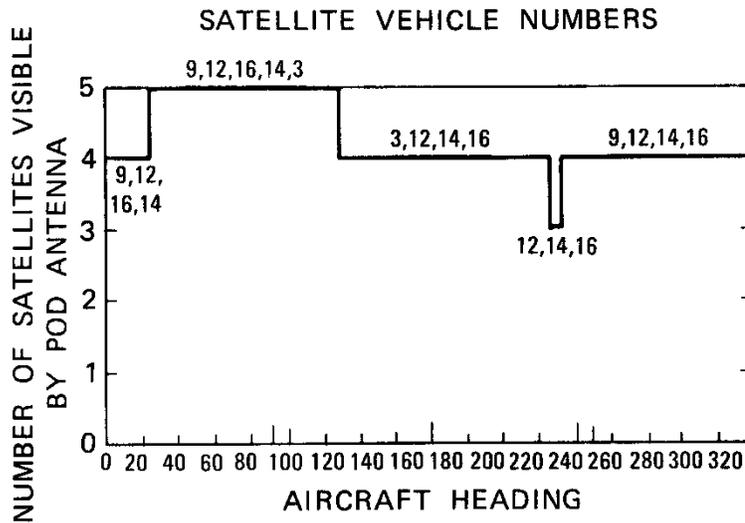
**Figure 10 - F-14 Wings-Level GPS Satellite Blockage Estimations as a Function of Aircraft Heading**
