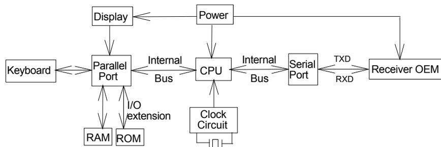
Figure1. The Navigation System Architecture
