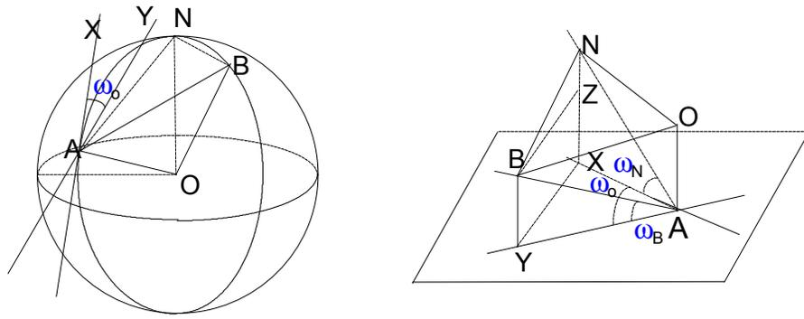
Figure 3. The spherical and plane diagram of the heading
