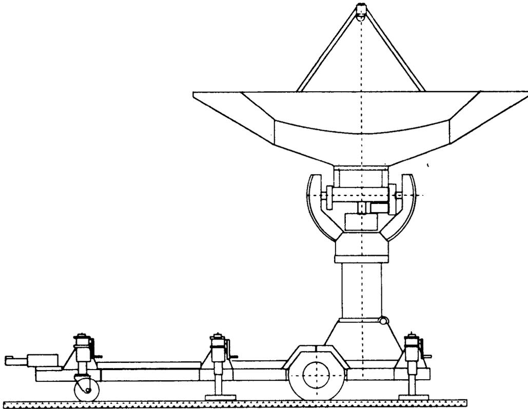
**FIG. 4: 4.3-METER X-Y MOBILE RECEIVE TERMINAL**
