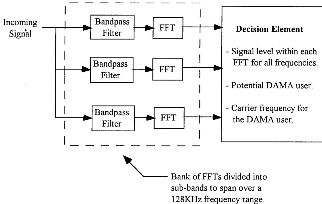
Figure 4 - Carrier Recovery Block Diagram for the DAMA Processor
