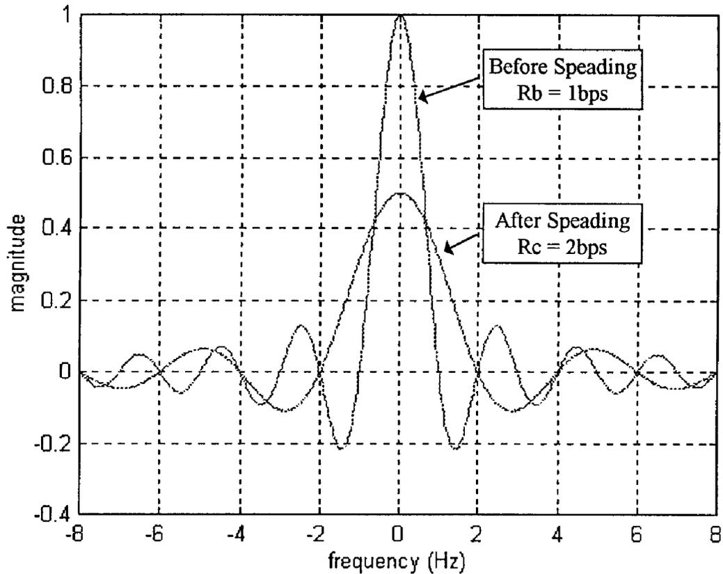
Figure 2 - Spectrum of a Digital Signal Before and After Spreading
