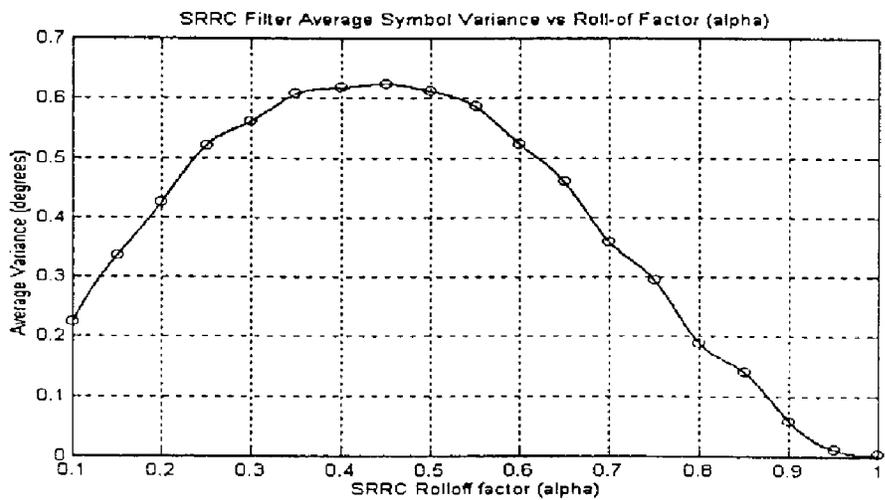
Figure 9 - SRRC: Average Symbol Variance vs Roll-off factor ( $\alpha$ )
