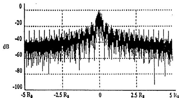
Figure 2 - Power Spectra: Output of SSPA at Saturation Level (No Baseband Filtering)
