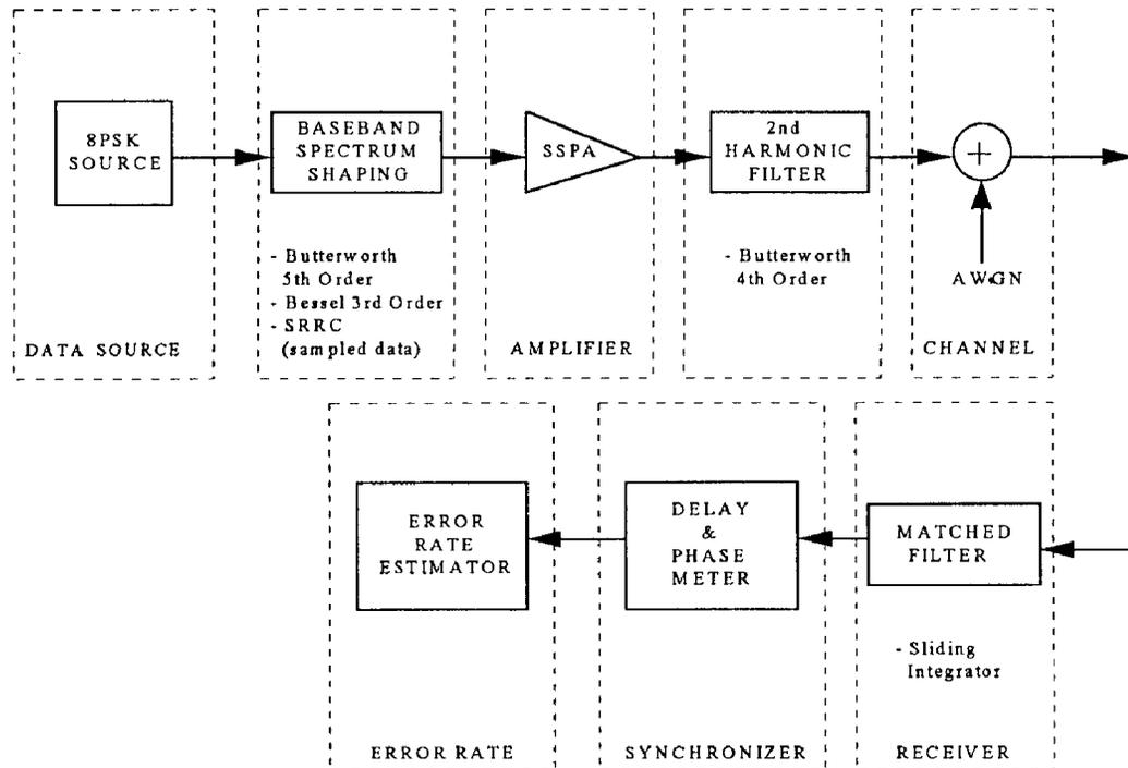
Figure 1 - Simulation Block Diagram
