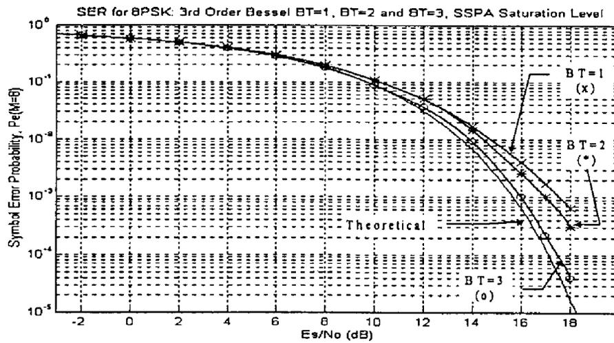
Figure 5 - SER for 8PSK: 3rd Order Bessel BT = 1, 2 and 3
