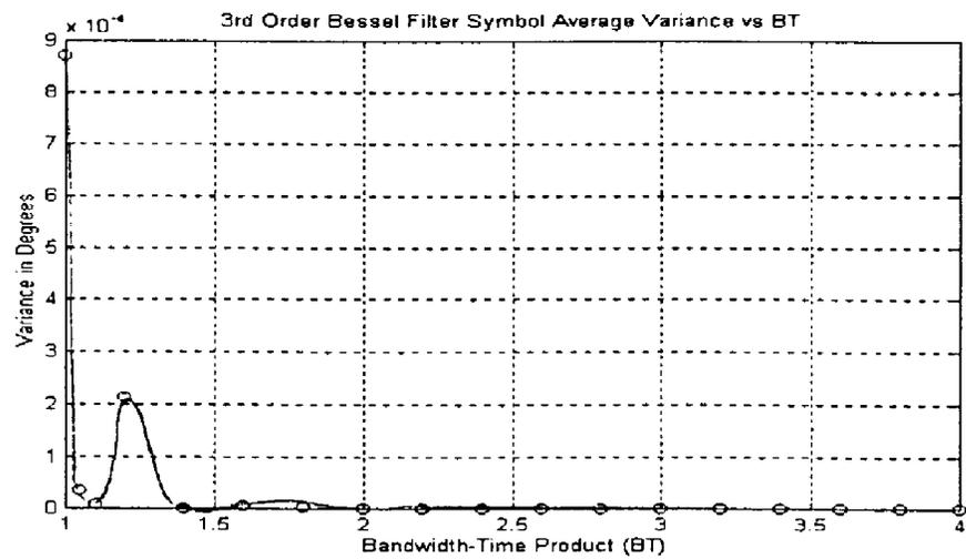
Figure 8 - 3rd Order Bessel Filter: Average Symbol Variance vs BT
