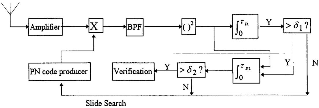
Figure 2 Block Diagram of Acquisition Circuit
