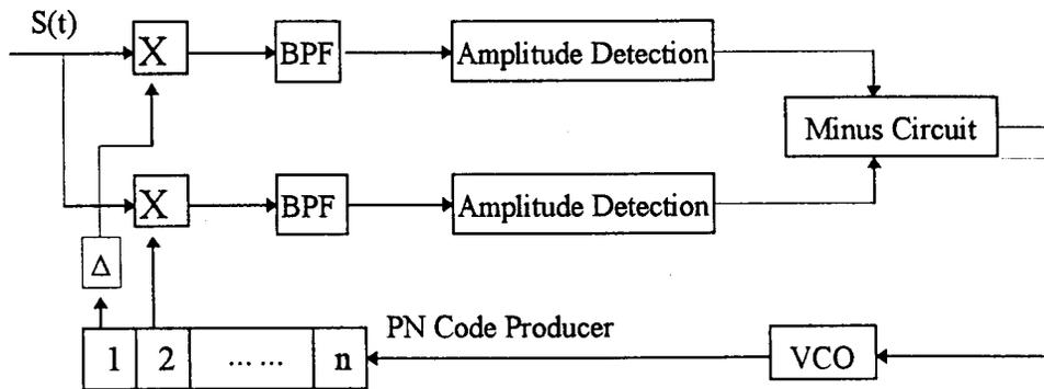
Figure 3 Block Diagram of Delay Lock Loop
