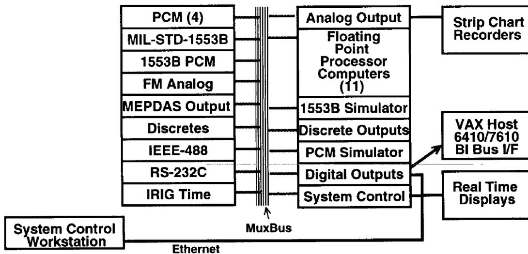
**Figure 3: Loral Pro 550 Data Acquisition System Block Diagram**
