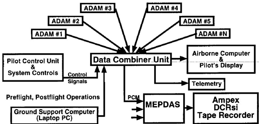
**Figure 2: Air Vehicle Data Acquisition System Block Diagram**
