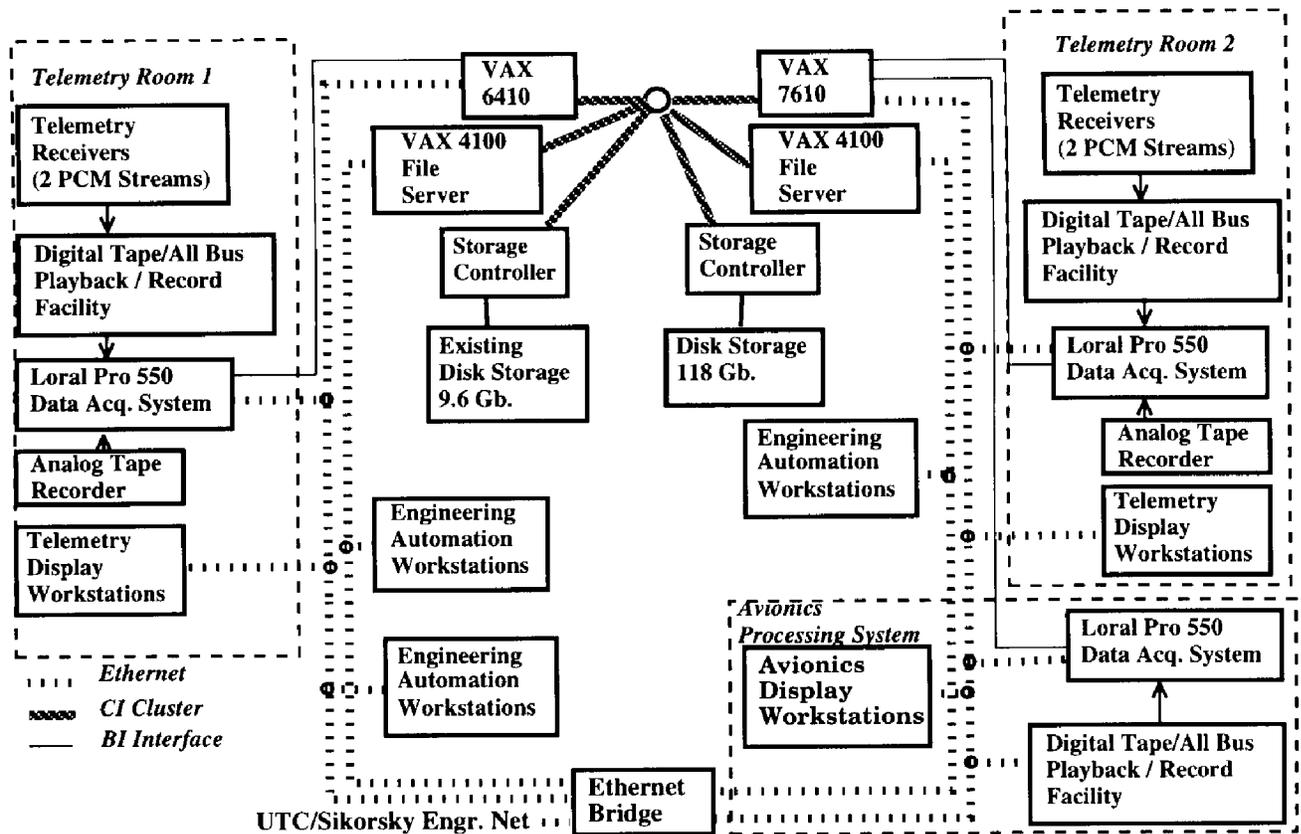
**Figure 5: ADAPS Ground Computer Facilities Block Diagram**
