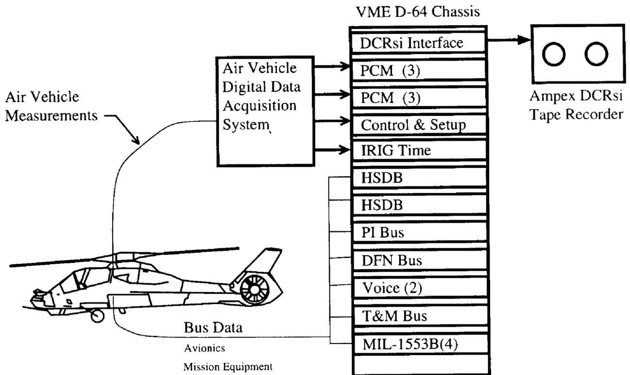
**Figure 1: Airborne Recording System Block Diagram**
