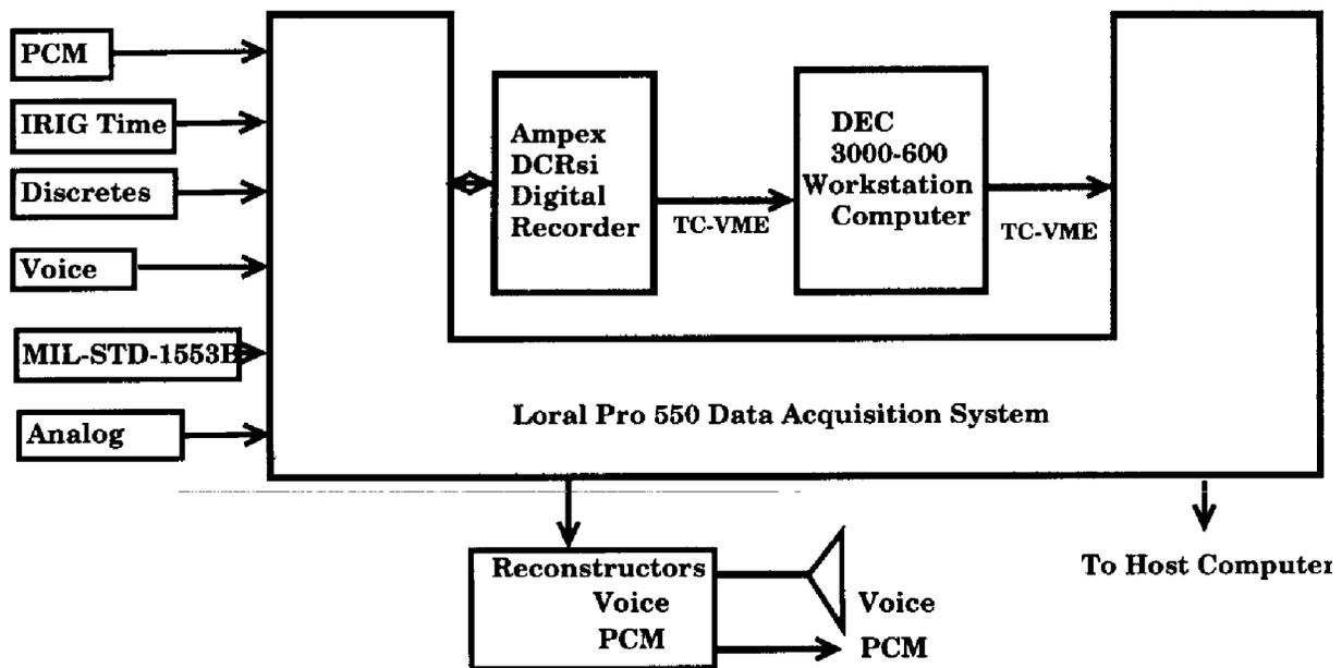
**Figure 4: MEPDAS Recording System Playback Block Diagram**
