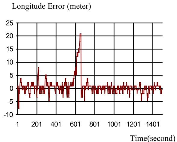
Figure 4 Longitude Error After DGPS
