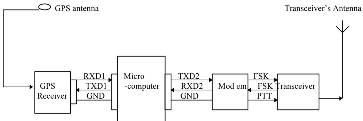
Figure 2 The movable station's architecture
