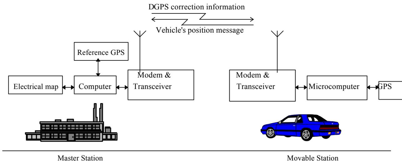
Figure 1 The System's Architecture
