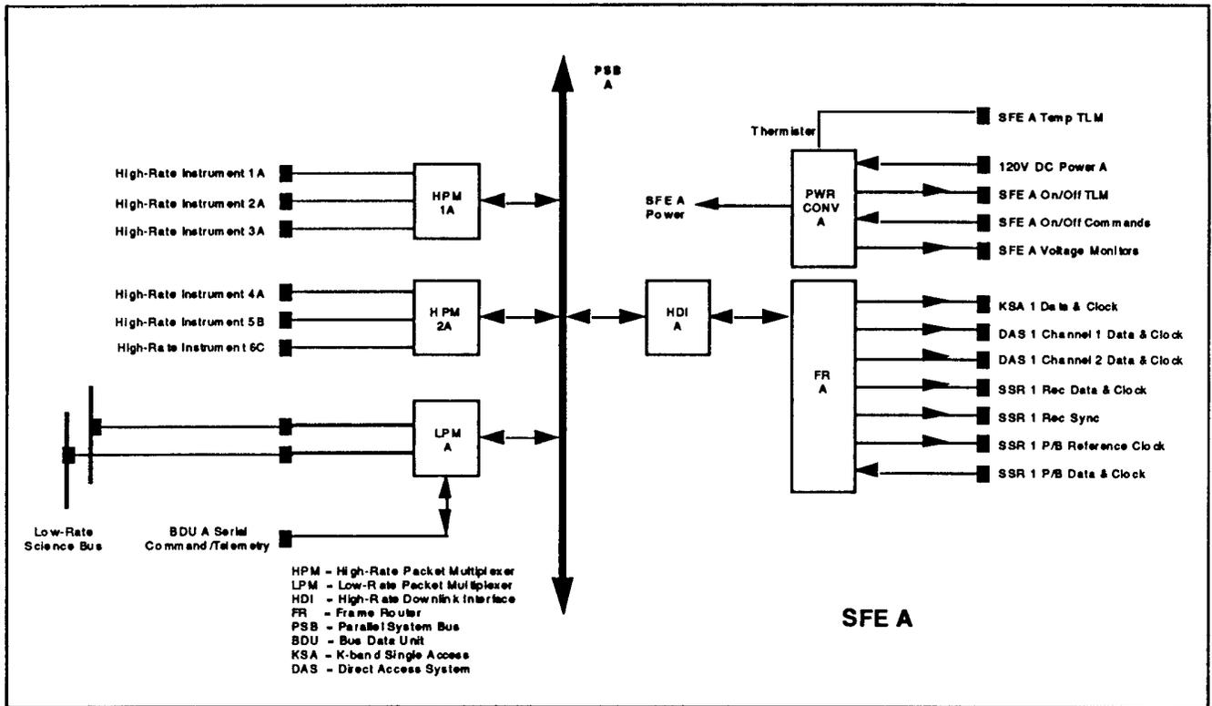
Figure 3: Block Diagram of the SFE
