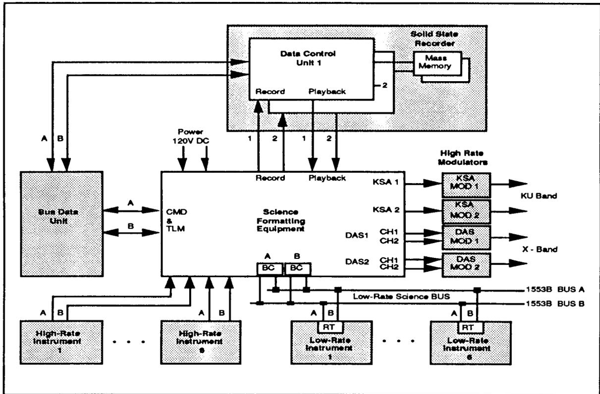
Figure 1: Block Diagram of the Science Telemetry Section of the EOS-AM1 Spacecraft
