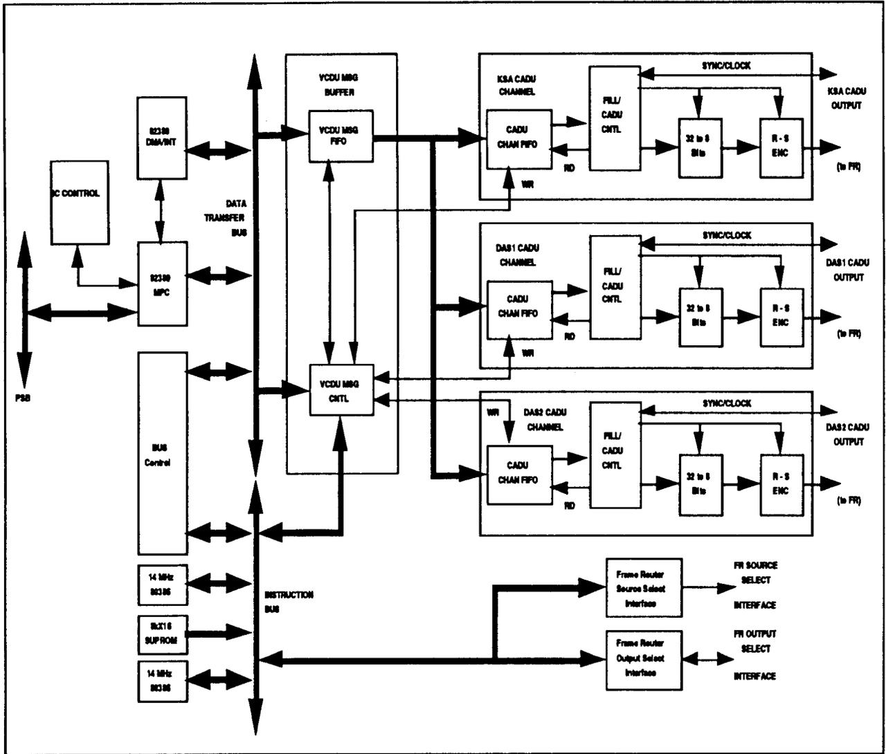
Figure 6: Block Diagram of the High-rate Downlink Interface Card
