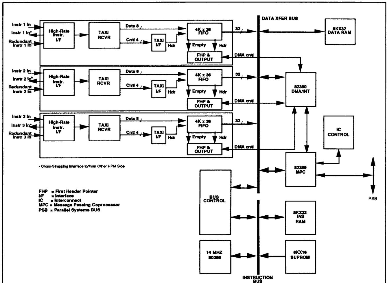
Figure 4: Block Diagram of the High-rate Packet Multiplexer Card
