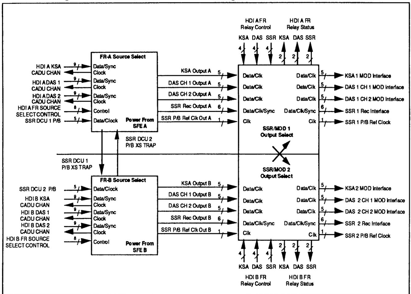
Figure 7: Block Diagram of the Frame Router Card
