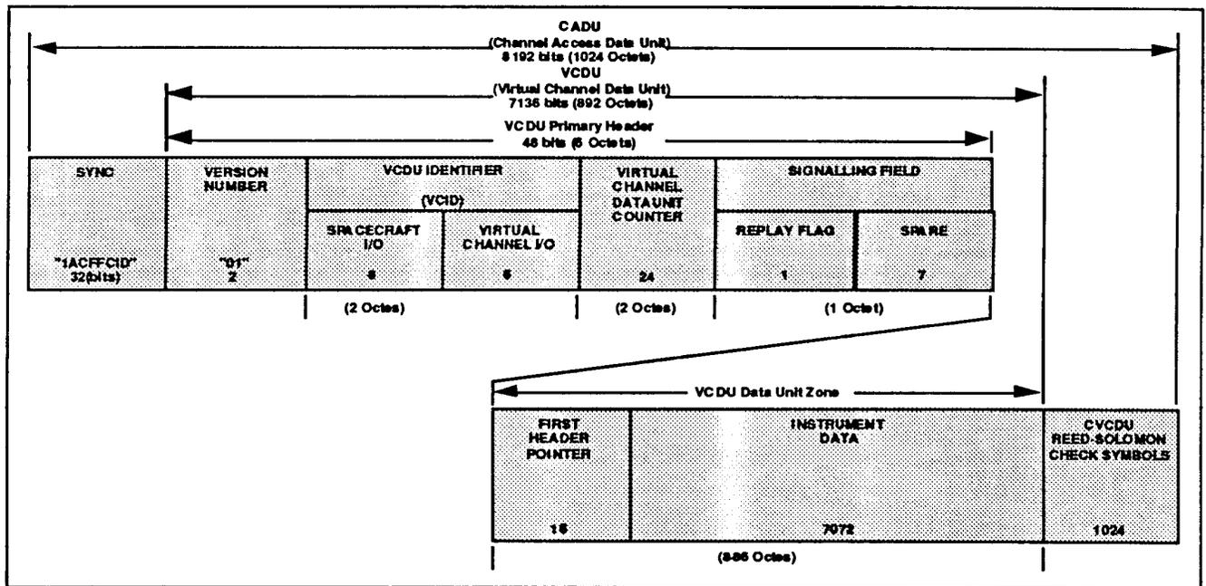
Figure 2: CCSDS Science Telemetry Frame Format
