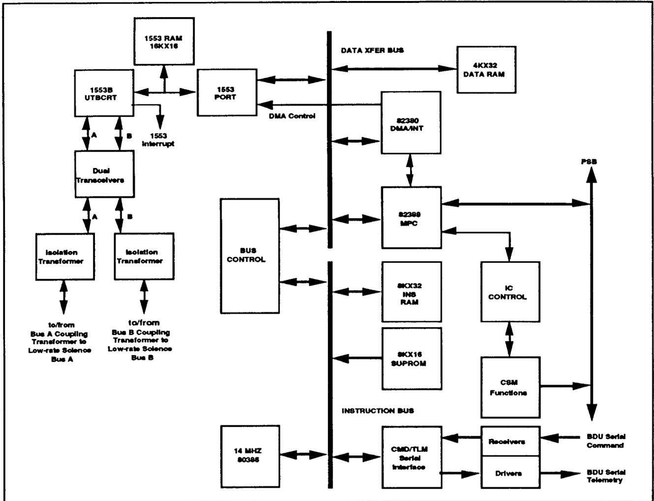
Figure 5: Block Diagram of the Low-rate Packet Multiplexer Card
