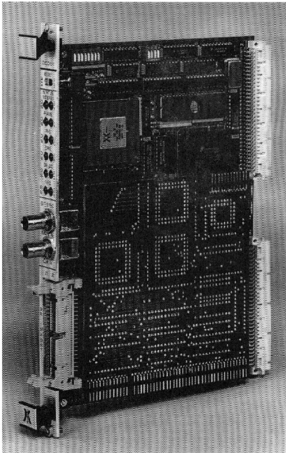
Figure 4 DEC012 Baseband Decoder Module, 3/4 View
