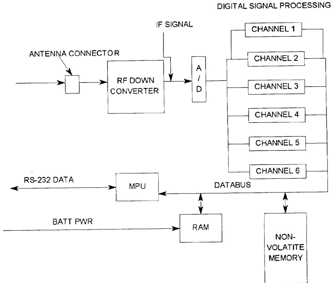
Figure 2. GPS Receiver Module Functional Block Diagram
