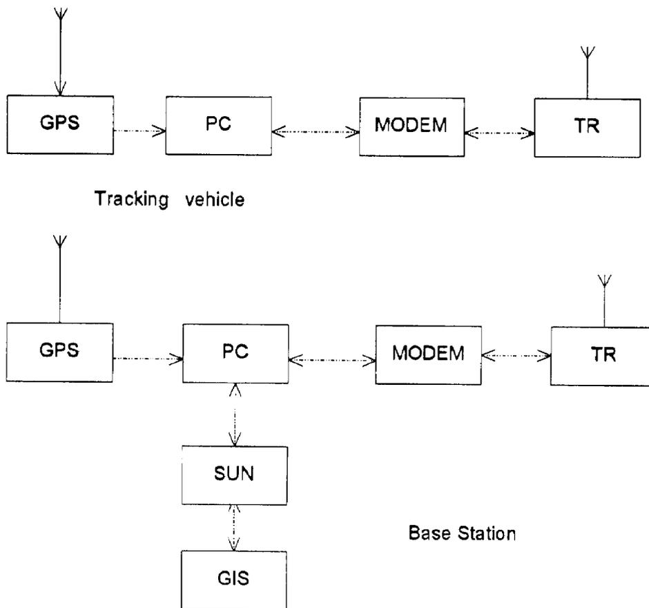
Figure 1. Block diagram of SCADA
