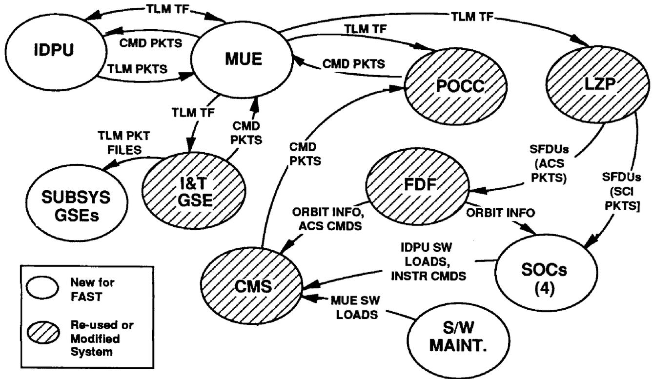
**Figure 4: FAST System-wide CCSDS Data Flow**
