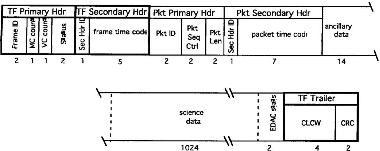
**Figure 3: FAST Transfer Frame with Science Packet**
