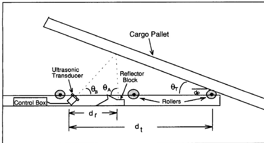
Figure 2. The Ultrasonic Angular Measurement System
