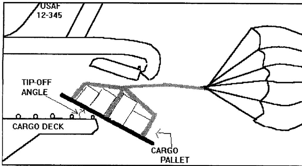
Figure 1. Cargo Pallet Extraction from an Aircraft
