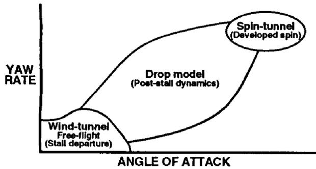
Figure 1. High AOA Test Technique
