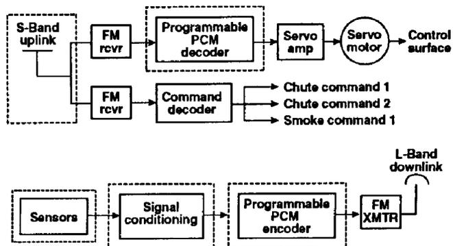
Figure 6. Airborne System Upgrade
