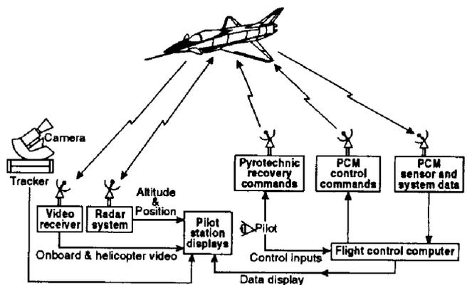
Figure 4. Overall Operation of Drop Model
