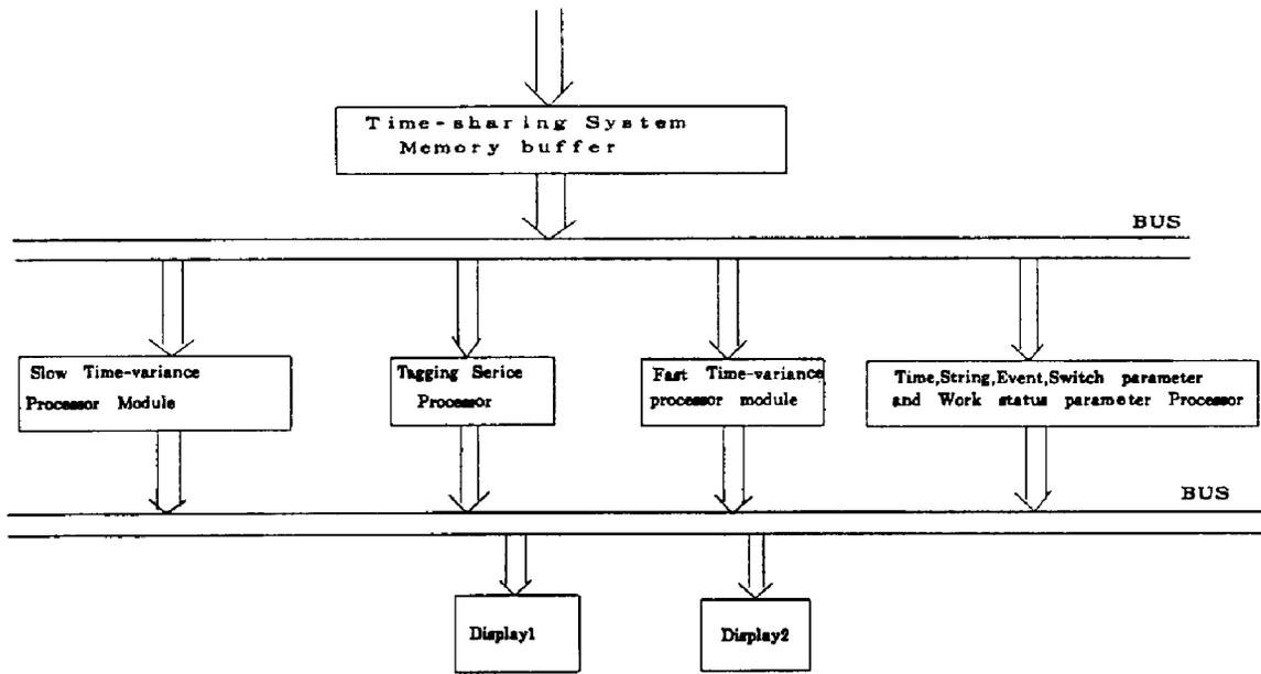
Figure 2. Time-sharing Processing Architecture
