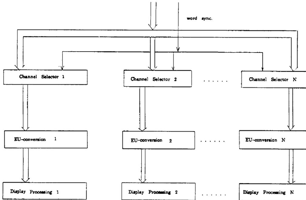
Figure 1. Multiple-channel Processing Architecture
