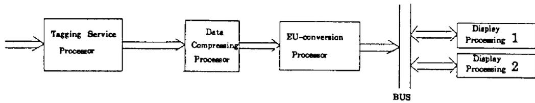
Figure 3. Pipeline Processing Architecture
