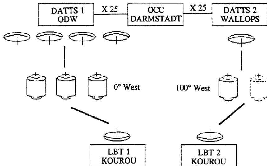
Fig. 4: MRS configuration for Meteosat and NOAA support
