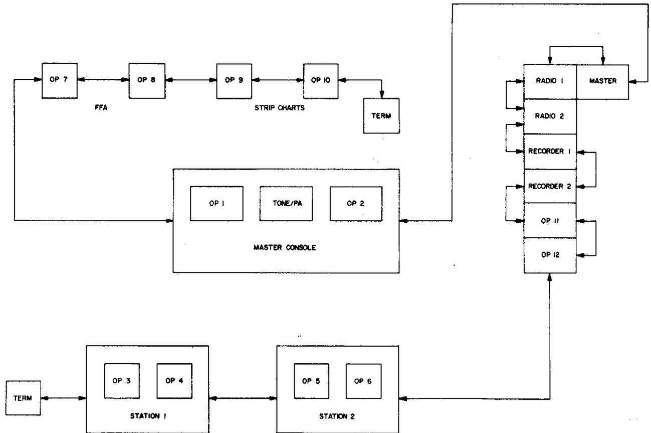
**Figure 5: FTCR Communication System Configuration**
