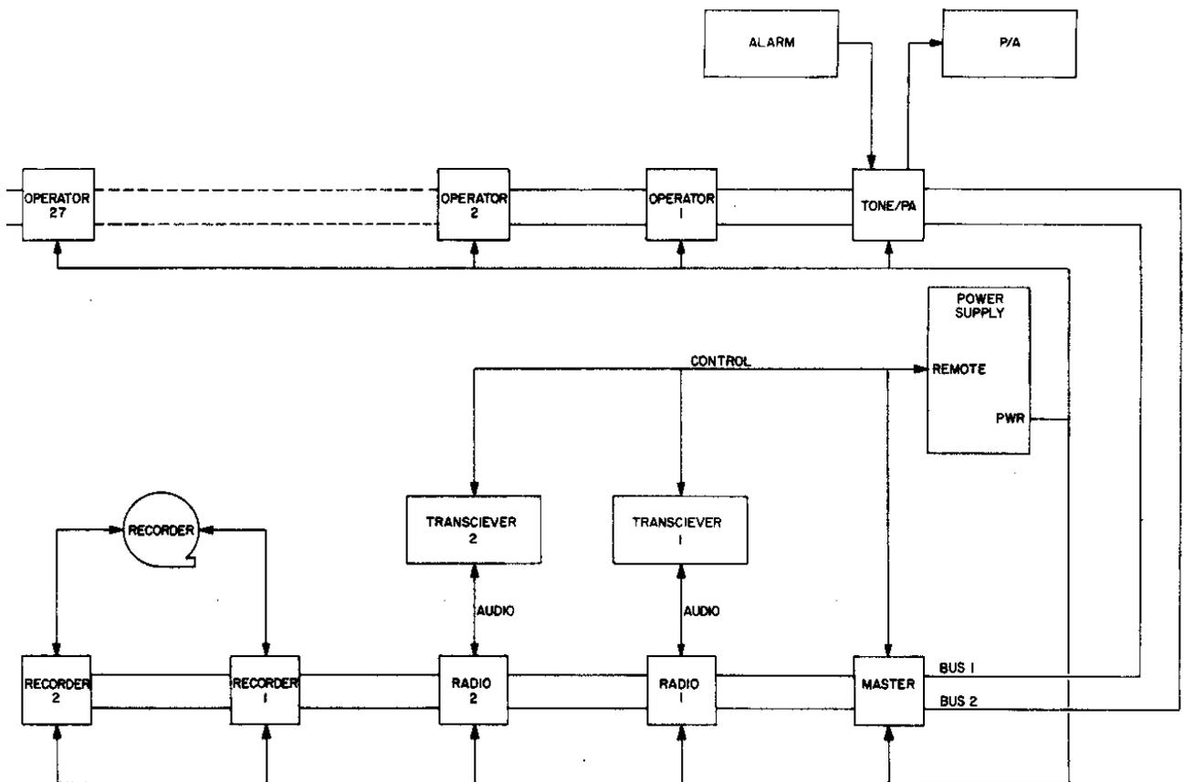
**Figure 4: Digital Communication System Block Diagram**
