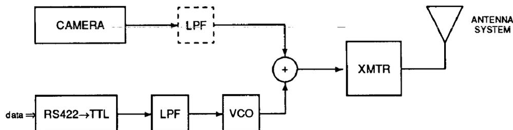
Figure 1: Block Diagram, Sending End
