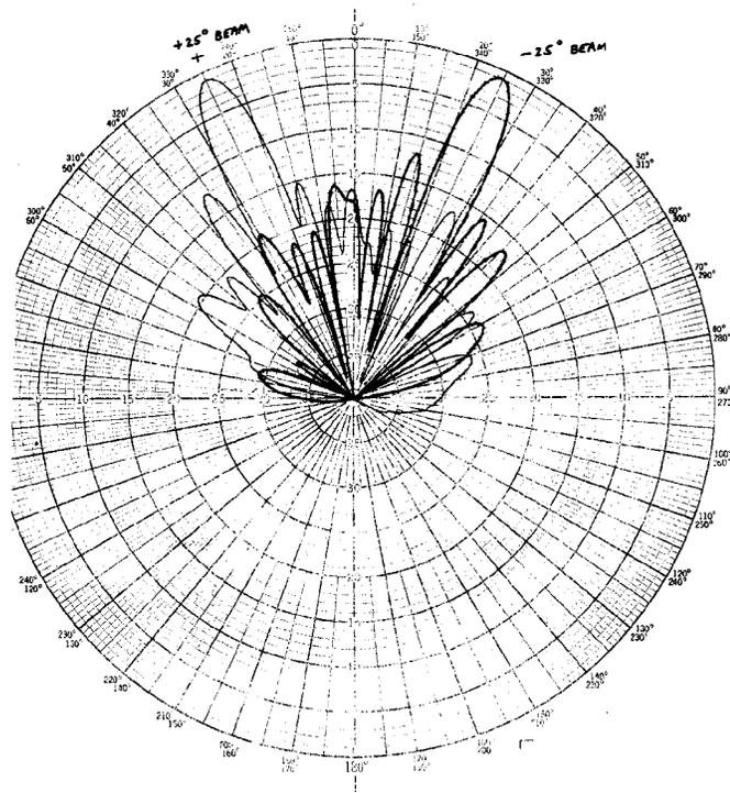
**FIGURE 11. ELEVATION SCAN BEAMS  $\pm 25$  DEGREES**
