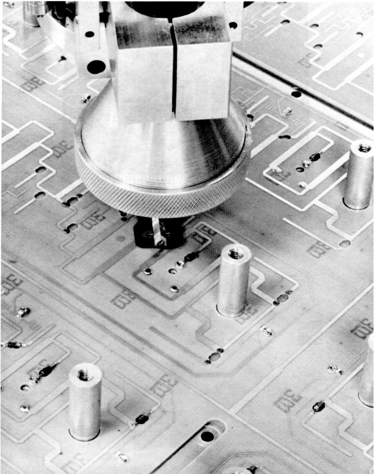
**FIGURE 6. ROBOTIC DIODE INSTALLATION**
