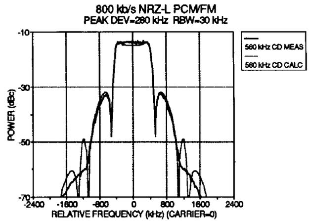
Figure 4 - PCM/FM with CD Filter.
