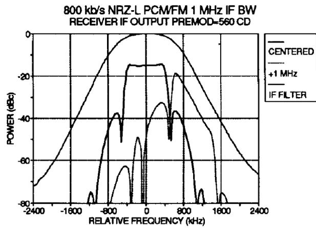
Figure 15 - Adjacent Channel (FM, +1 MHz).
