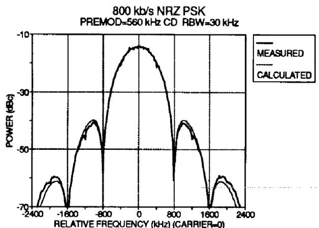
Figure 12 - PSK with CD Filter.
