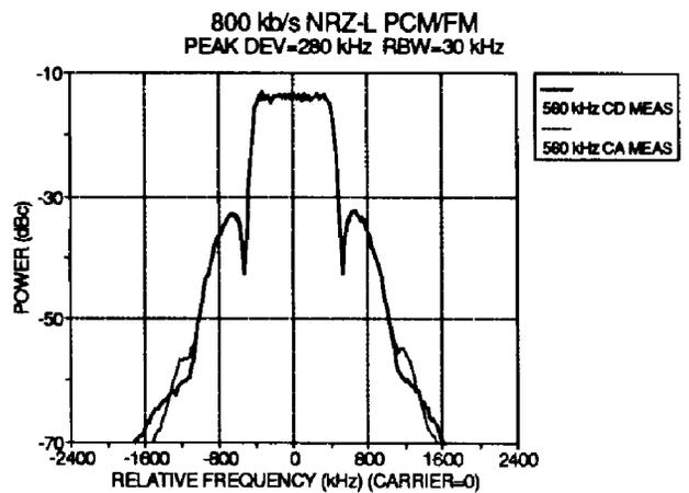
Figure 8 - PCM/FM with CD and CA Filters.
