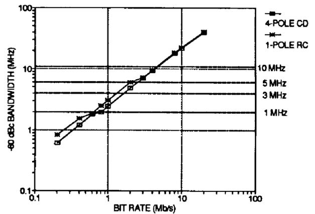
Figure 10 - PCM/FM -60 dBc Bandwidth.
