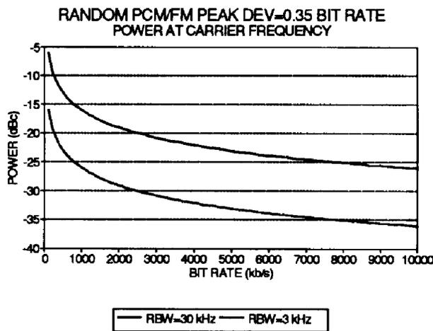
Figure 9 - PCM/FM Center Frequency Power.
