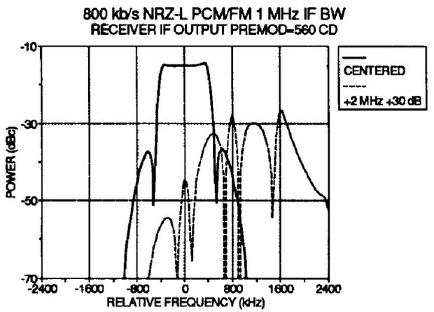
Figure 16 - Adjacent Channel (FM, +2 MHz).
