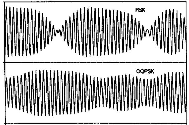
Figure 14 - PSK and OQPSK Envelopes.
