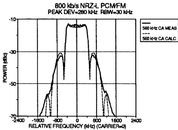
Figure 7 - PCM/FM with CA Filter.
