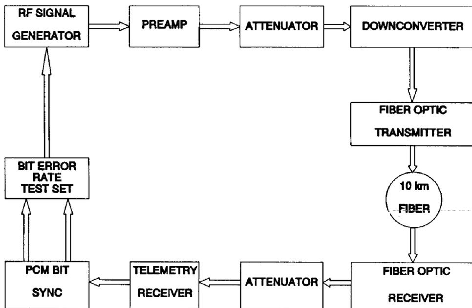
Figure 5. Test Setup for Bit Error Rate Test.
