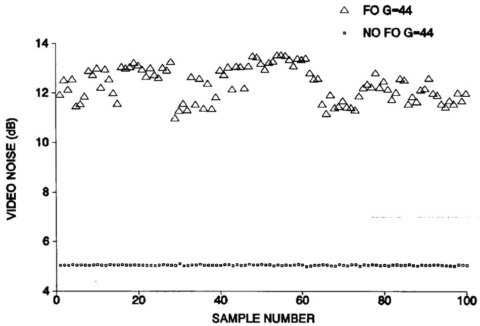
Figure 3. Receiver Video Noise Level Instability.
