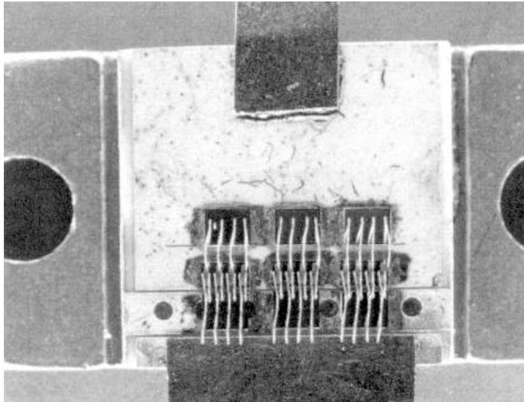
**FIGURE 1. PHOTO OF 50W 1700-1850 MHz DEVICE**
