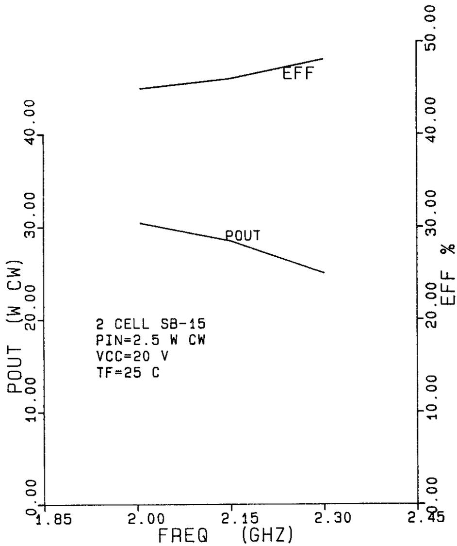
**FIGURE 5 POWER OUTPUT AND EFFICIENCY OF 2000 - 2300 MHZ DEVICE**
