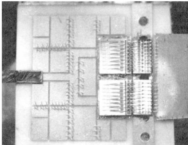
**FIGURE 4. PHOTO OF 25W 2000 - 2300 MHZ DEVICE**
