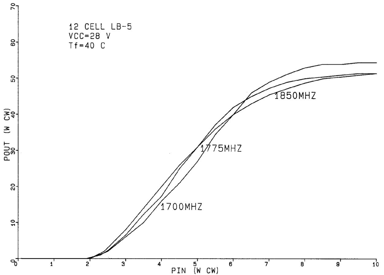
**FIGURE 2 TRANSFER CHARACTERISTIC OF 1700 - 1850 MHz DEVICE**
