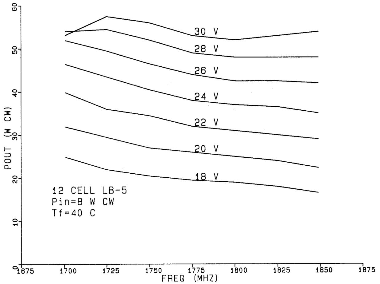
**FIGURE 3 VCC RESPONSE OF 1700 - 11850 MHZ DEVICE**
