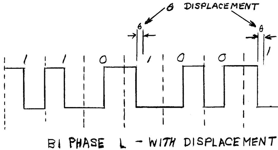
FIGURE 4 EDGE DISPLACEMENT
