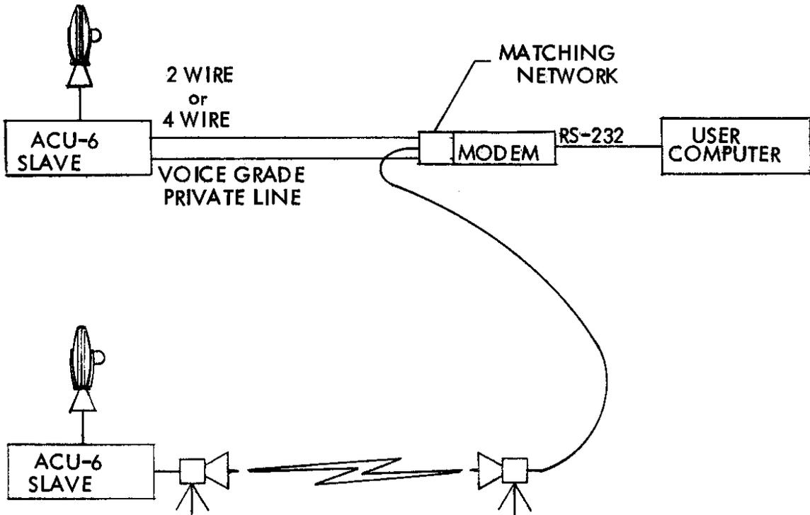
**FIGURE 4 ACU-6 NETWORK USING EXISTING
