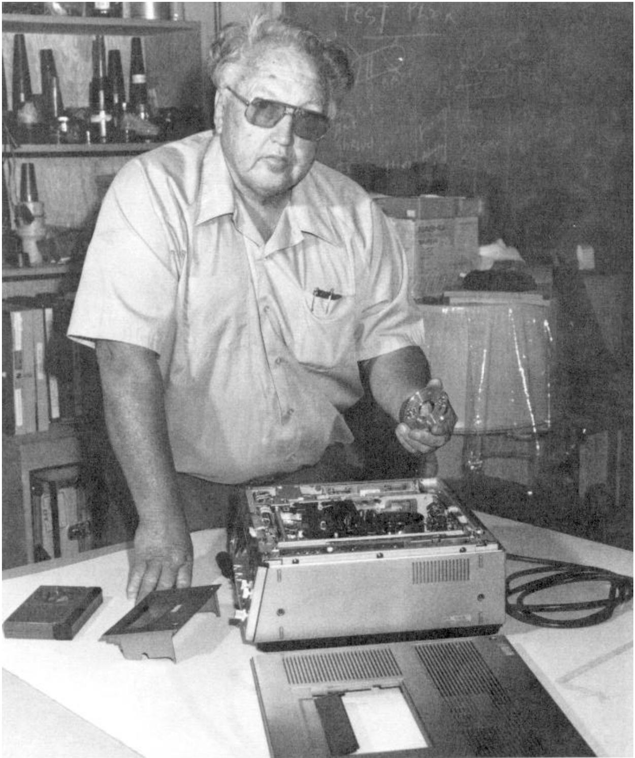
FIGURE 5. AUTHOR HOLDING HEAD ASSEMBLY, SHOWING SIZE AND EASE OF REPLACEMENT.
