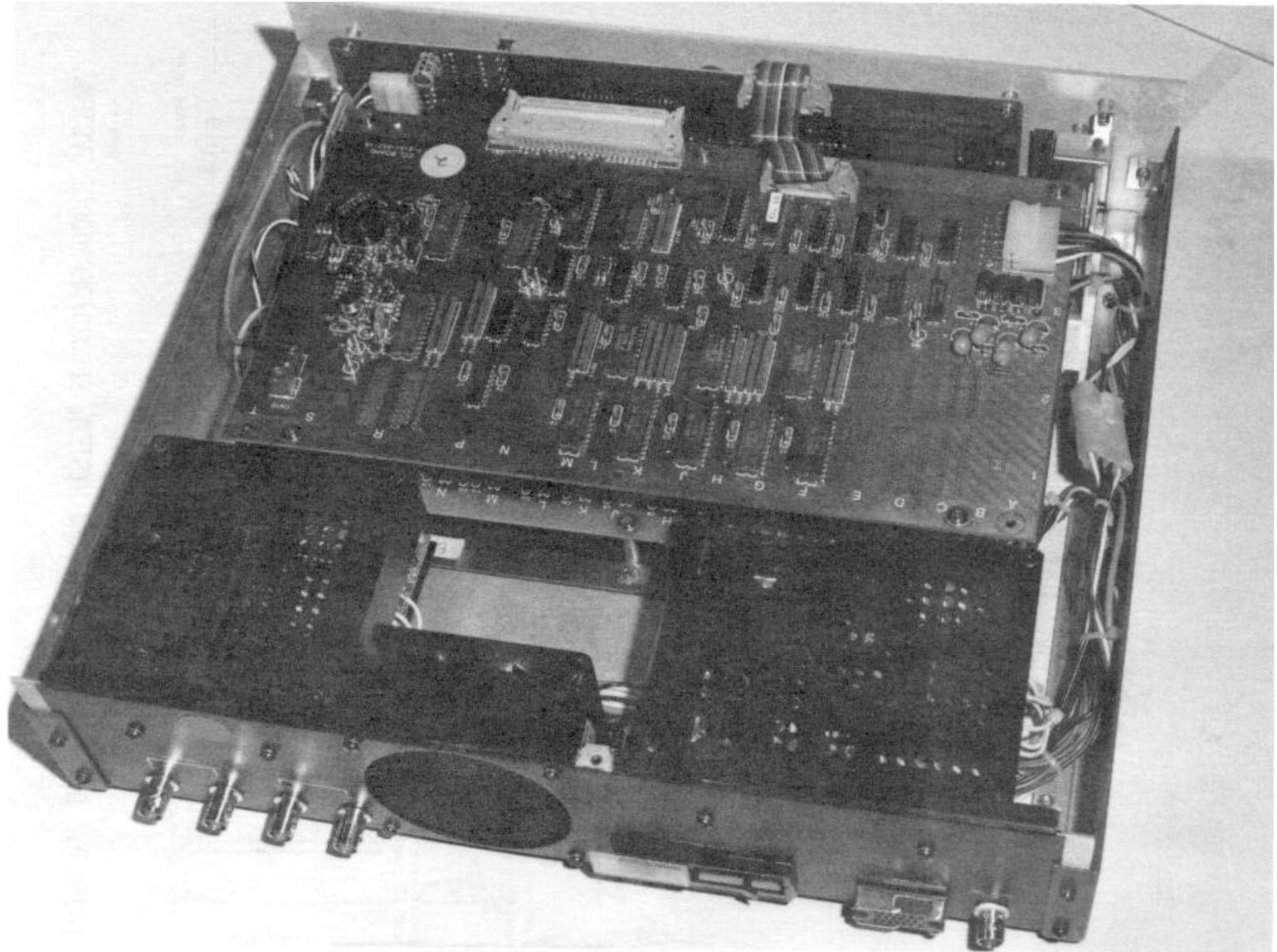
FIGURE 6. BASIC BOARD, DATA CONVERSION/TLM ADAPTER.
