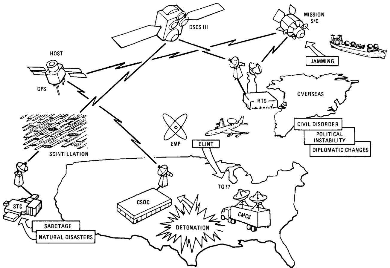
**FIGURE 1 SURVIVABILITY/INTEROPERABILITY CONCEPTS.** The threats to space resources and their ground support elements are illustrated. The alleviation of the threats by cross links to CONUS, improved signal structure, mobile resources, and elimination of single nodes are indicated.
