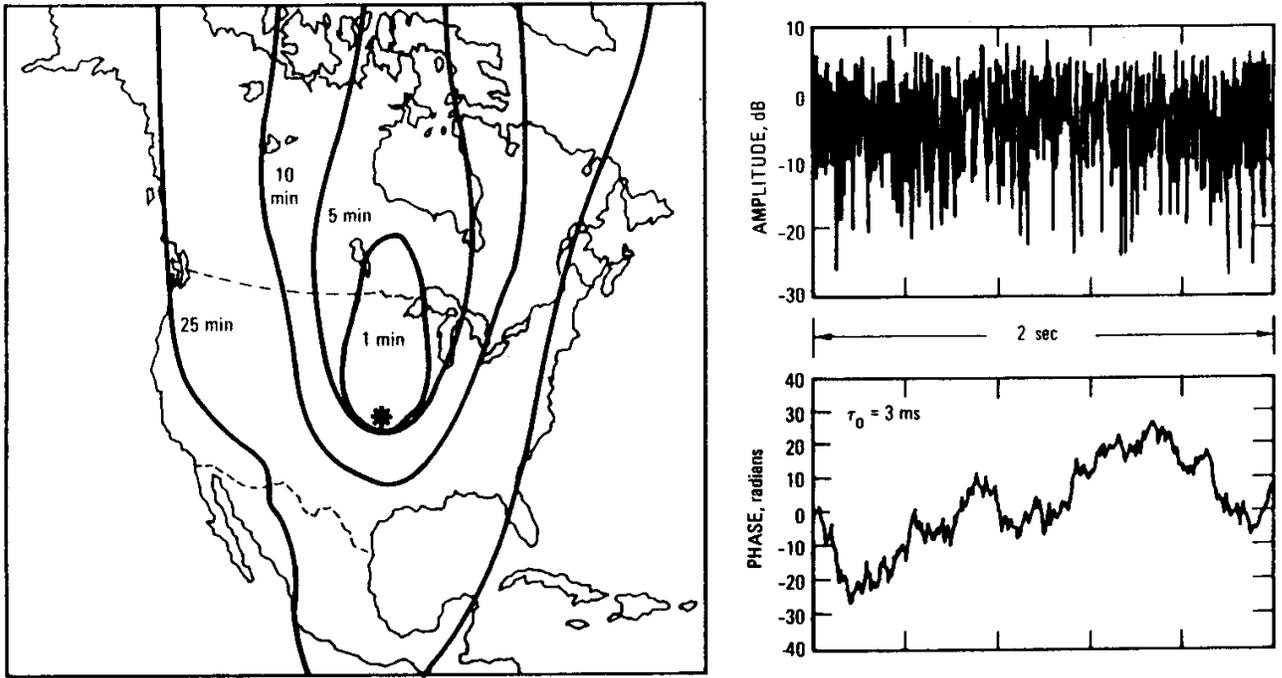
**FIGURE 2 SCINTILLATION-S BAND.** Exoatmospheric nuclear explosions radically disturb the upper atmosphere and ionosphere for many hours causing serious phase and amplitude distortions of spacecraft data links.
