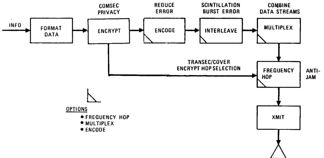
**FIGURE 3 STANDARD AND ATT&C FUNCTIONS.** A typical functional flow of data through an ATT&C station uplink.
