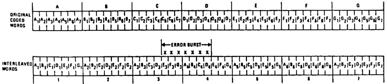
**FIGURE 8 INTERLEAVING.** Interleaving data prevents the error burst from propagating when used with the previously described convolutional coding error correction technique.
