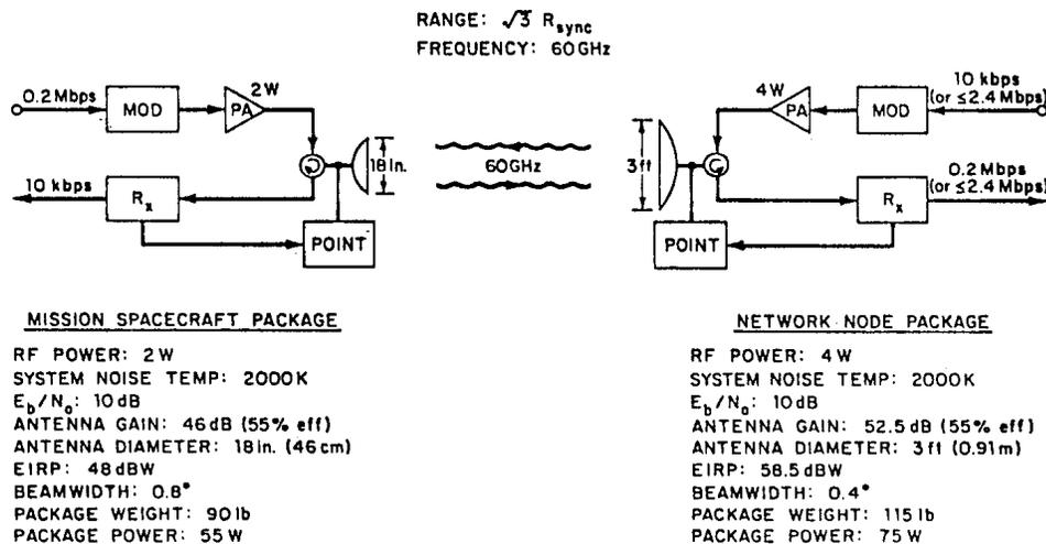
Technology assumptions for 60 GHz TTC access link (200 kbps). As a cross-orbit trunk, the network node package can handle 12 TTC channels (2.4 Mbps) bi-directionally.
