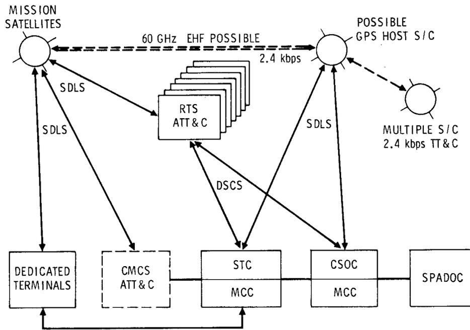
**FIGURE 10 AFSCN WITH ADVANCED TT&C CIRCA 1990.** The key items being implemented are the crosslinks to a host satellite and the retrofiting of an ATT&C EHF system into the common mobile control systems for high AJ capability and low probability of intercept.
