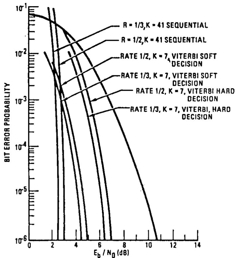
**FIGURE 7 VITERBI DECODER PERFORMANCE RATE 1/2 vs RATE 1/3.** A chart indicating the performance of various constraint lengths and possible rates of bit error Improvements.
