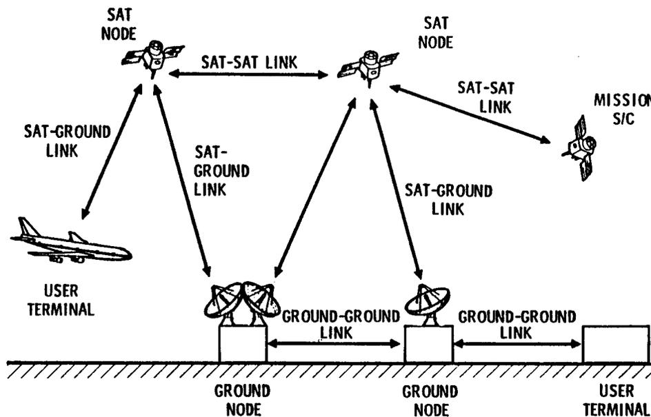
**FIGURE 4 GENERIC INTERNET LINKS.** Interoperable nodes and cross links are made possible using standardized networks and spacecraft.
