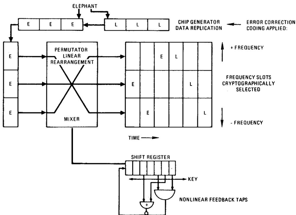
**FIGURE 5 CHIP GENERATION, PERMUTATION AND FREQUENCY HOPPING.** Frequency slots, assigned by a cypher key are used to assure future hops cannot be determined by an enemy thus providing transmission security (TRANSEC) antijam resistance, and low probability of intercept.
