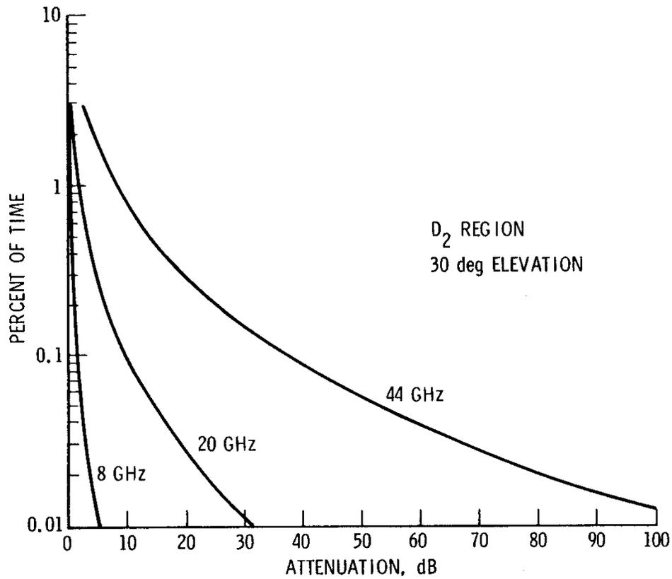
**FIGURE 9 RAIN ATTENUATION.** The outage from rain interference rapidly increases with frequencies above 10 GHz.
