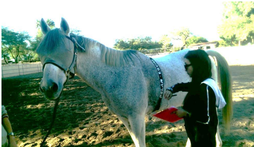
Figure 1.2: Depicts Polar Equine Heart Rate Monitor; the electrode transmitter is attached to a strap and is worn around the horse's abdomen; the wristwatch receiver is worn by the investigator.
