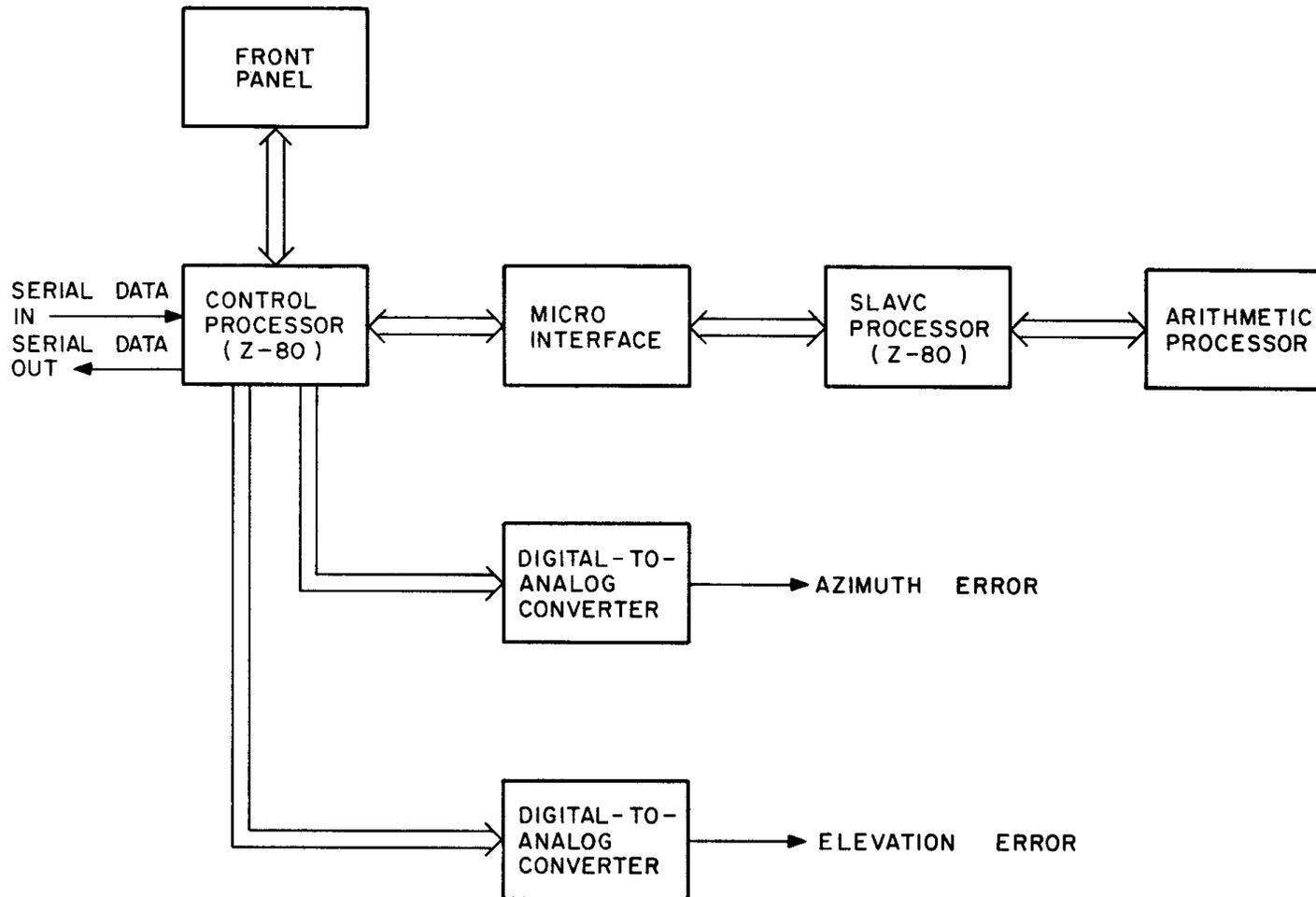
**FIGURE 7 TSI BLOCK DIAGRAM**
