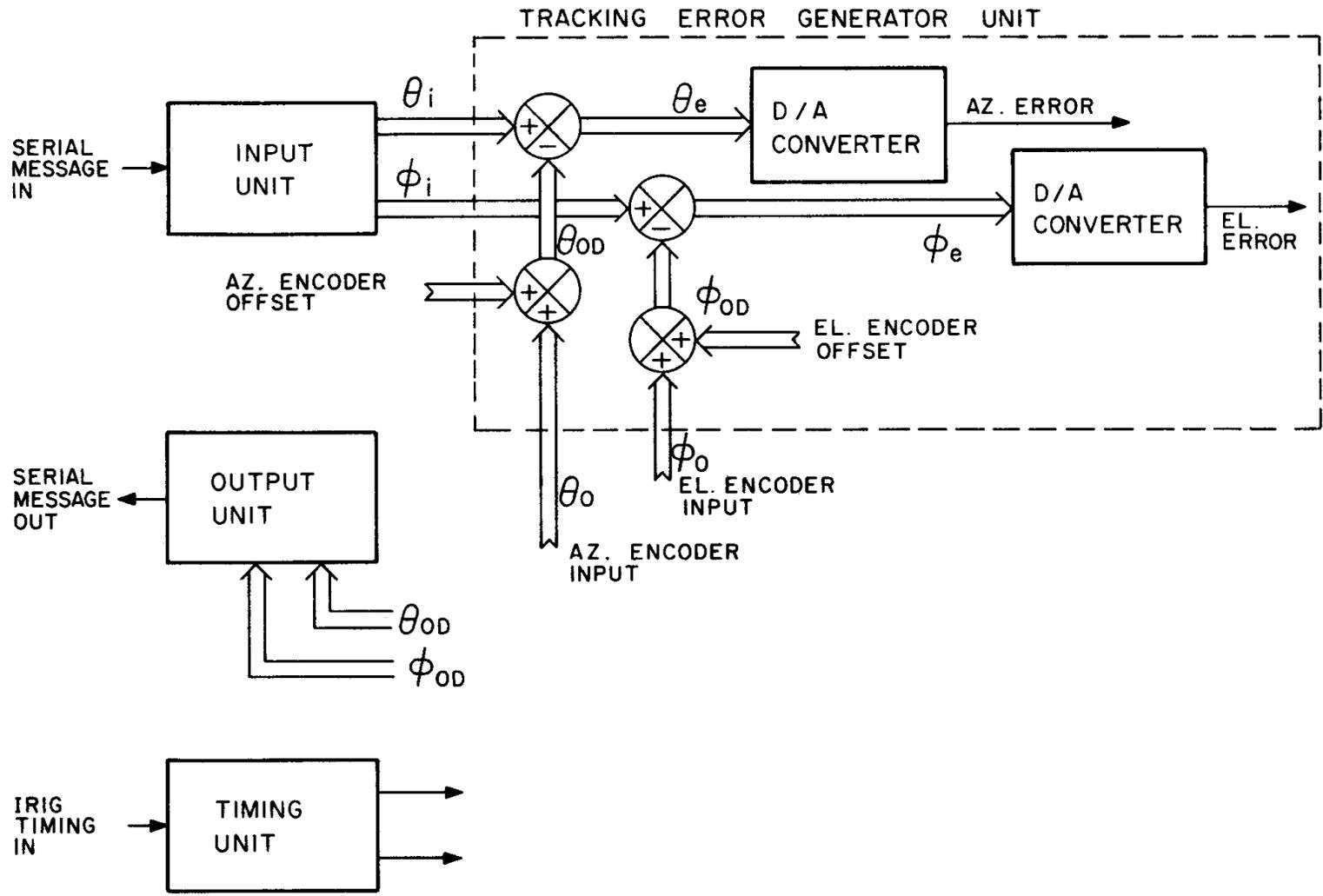
FIGURE 4 INSTRUMENT DATA CONVERTER
