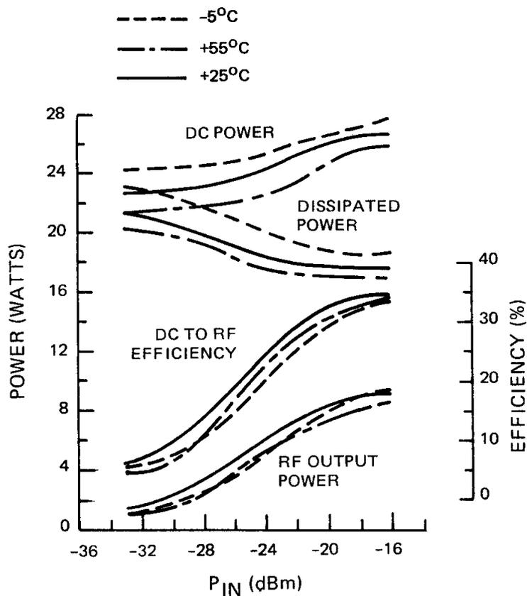
Figure 5. SSPA Power Distribution as a Function of Input Power and Temperature
