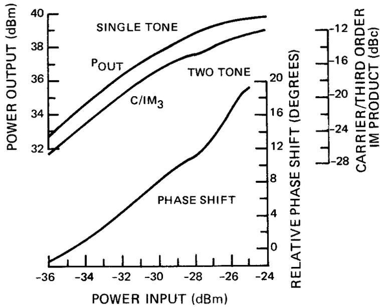
**Figure 3. SSPA Power and Phase Transfer Characteristics for a Single-Tone Input (Two-Tone C/IM<sub>3</sub> Characteristic Also Shown)**
