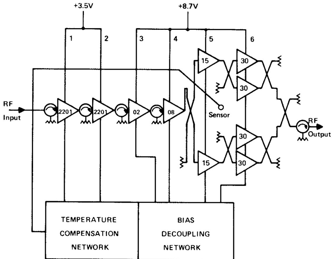
**Figure 1. SSPA Block Diagram**
