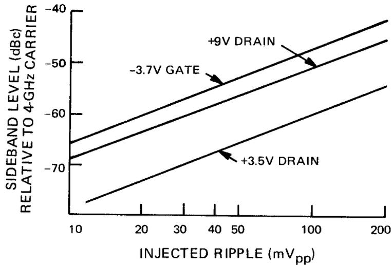
Figure 7. SSPA Ripple Sensitivity
