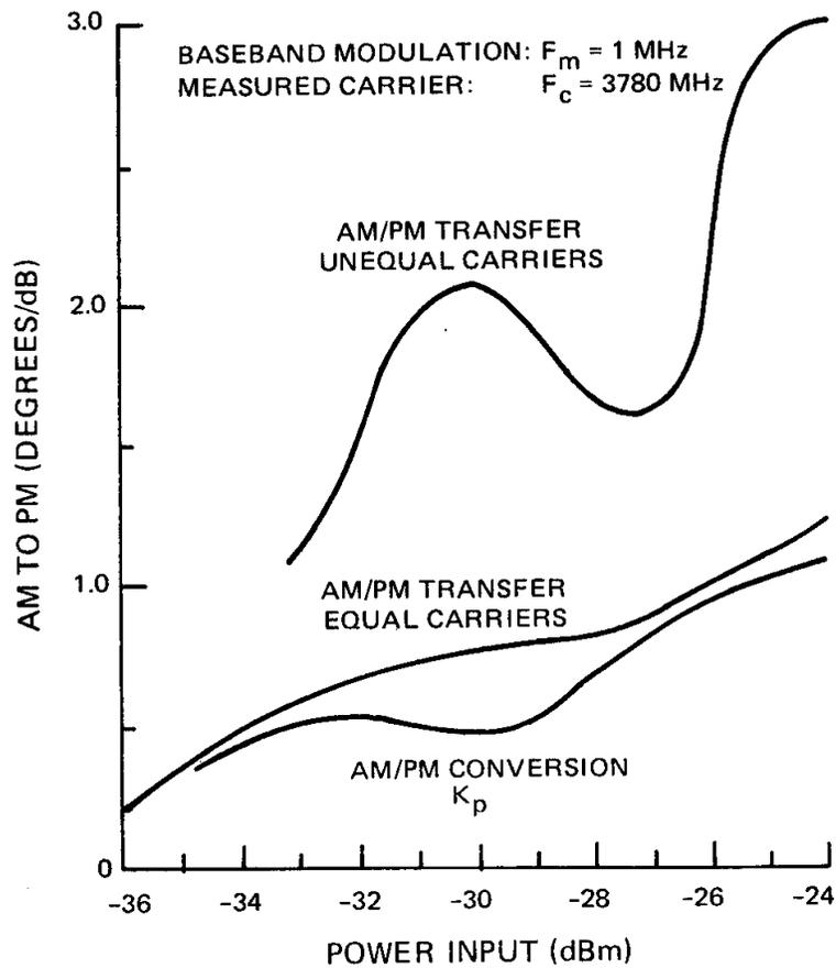
**Figure 4. AM-PM Conversion Coefficient ( $K_p$ ) and Transfer Coefficient ( $K_T$ )**
