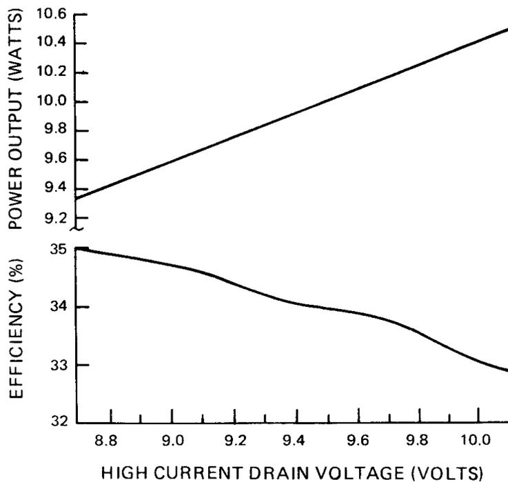
Figure 6. SSPA Power Output and Efficiency as a Function of Drain Voltage
