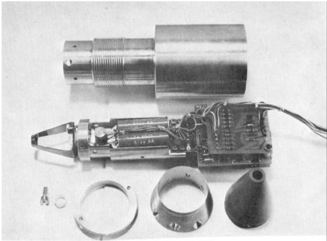
Fig 5: TM-M Series telemetry package Internal components.
