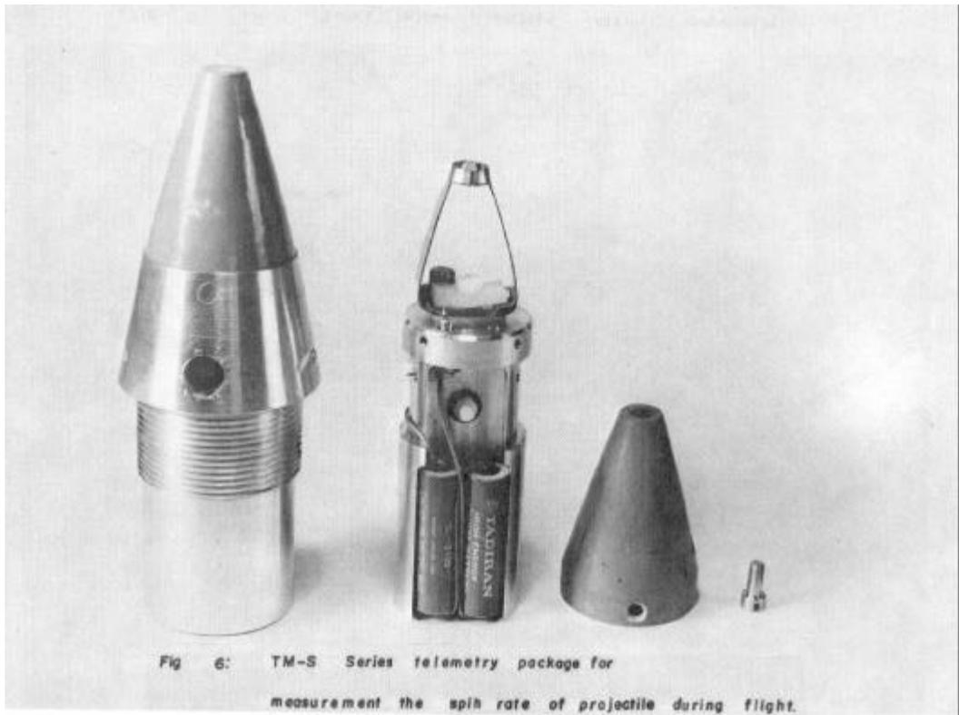
Fig 6: TM-S Series telemetry package for measurement the spin rate of projectile during flight.
