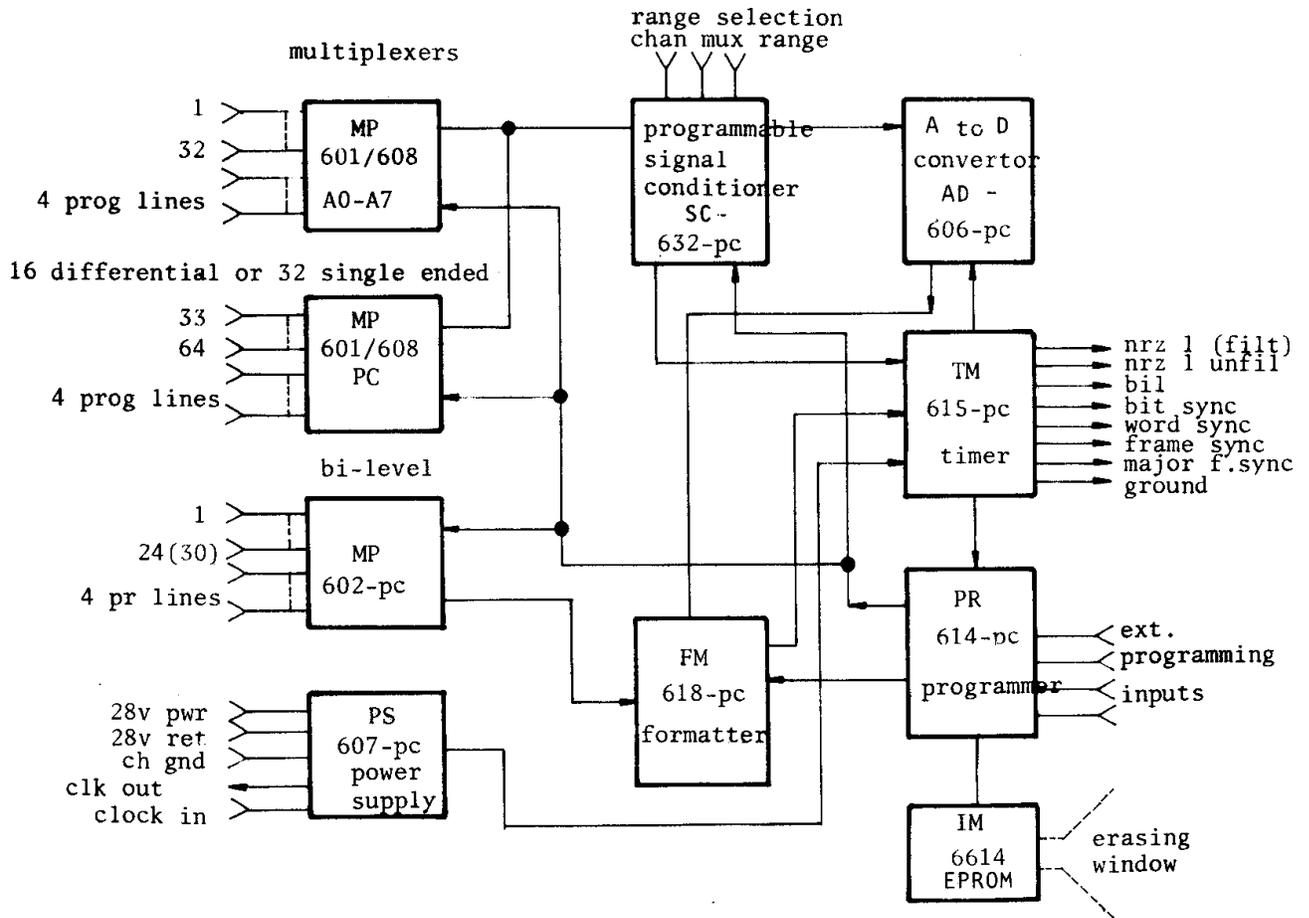
FIG. 12: PCM ENCODER FUNCTIONAL BLOCK DIAGRAM.
