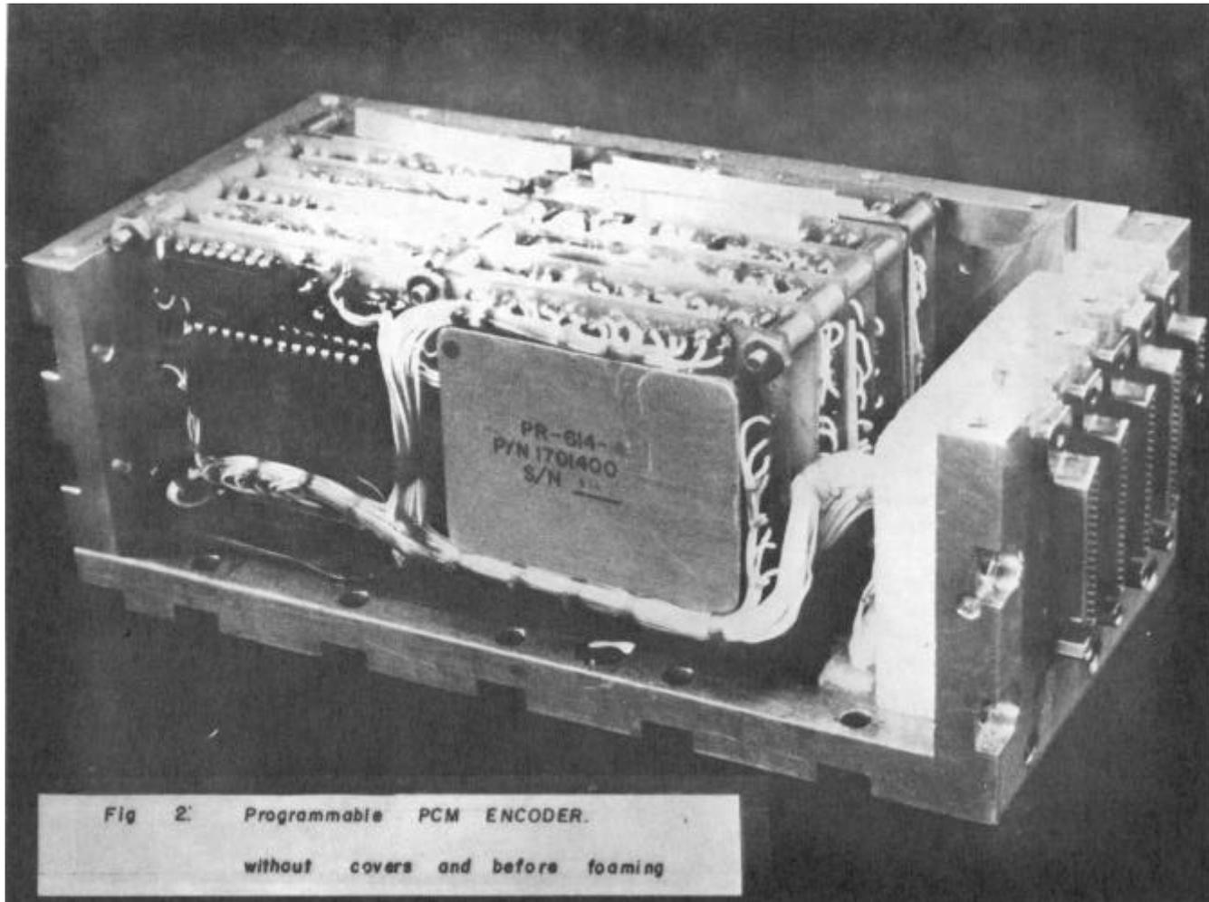
Fig 2: Programmable PCM ENCODER.
