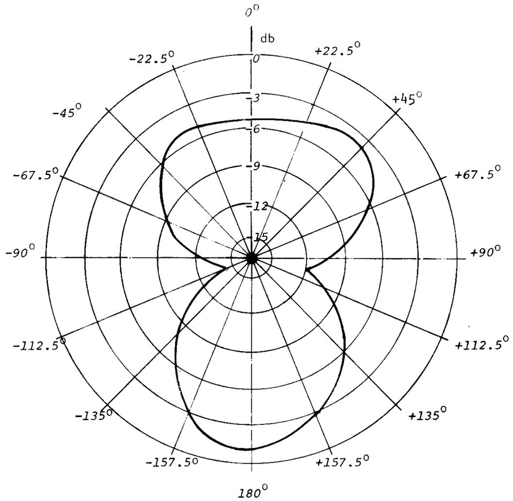
Fig 11 : Roll plane pattern of the transmitting antenna of TM-S and TM-M telemetry systems.
