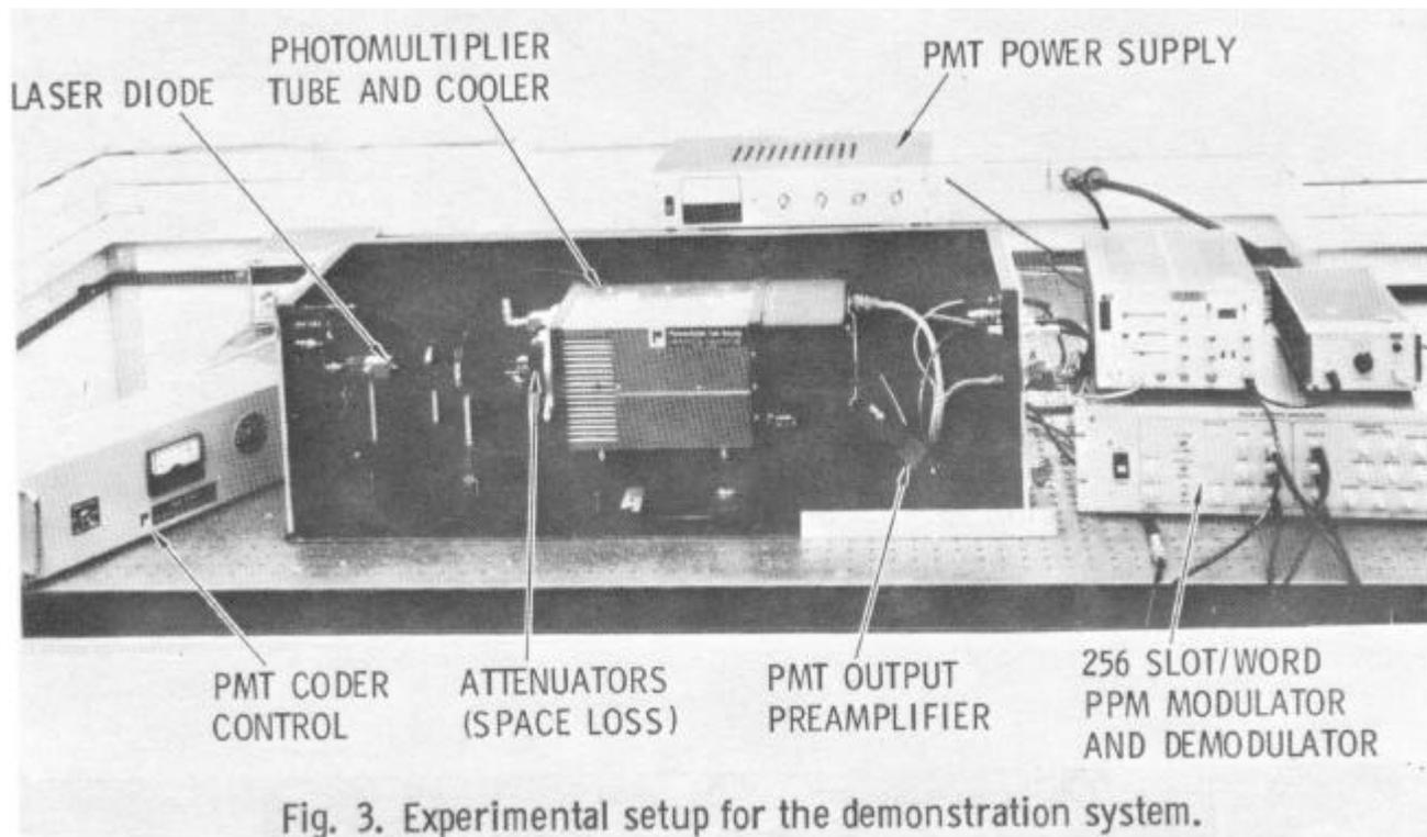
Fig. 3. Experimental setup for the demonstration system.
