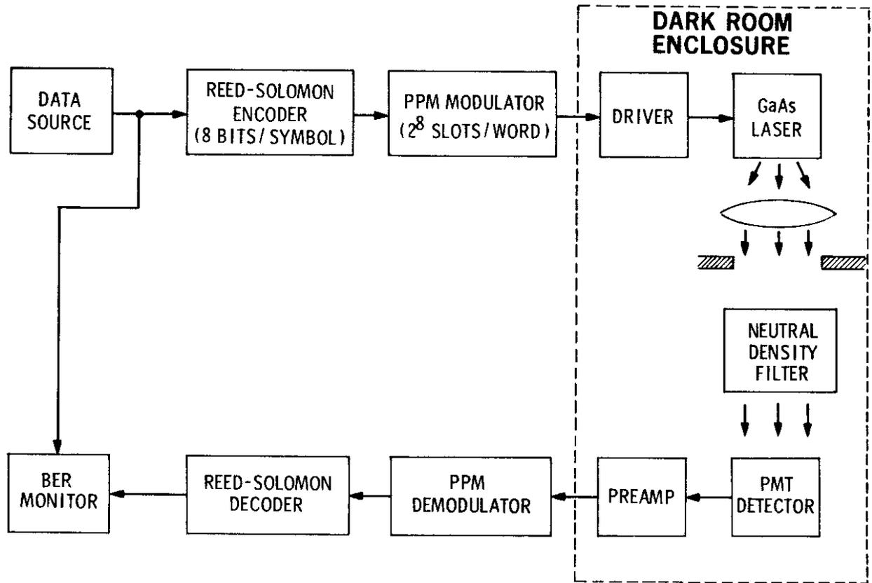
**Fig. 1. Block diagram of 2.5 bit/detected photon demonstration system.**
