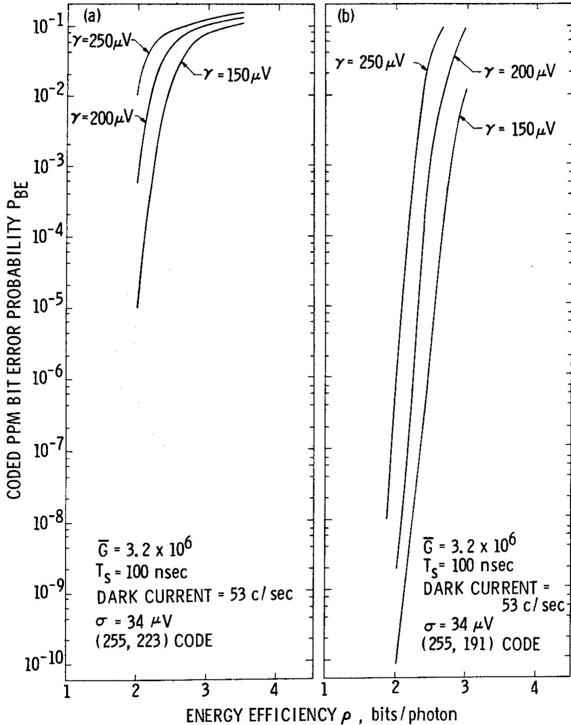
Fig. 2. Coded bit error performance for PMT gain of  $3.2 \times 10^6$  and 53 dark counts/ sec.: (a) (255, 223) rate 7/8 R-S code, (b) (255, 191) rate 3/4 R-S code.
