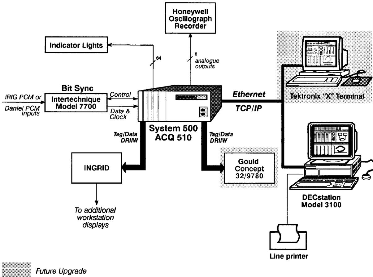
Figure 9. Loral Instrumentation System 500 at Dassault Istres
