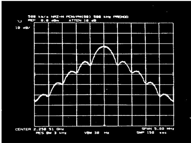
**Figure 2D. NRZ-M PCM/PM( $\pm 90^\circ$ )
