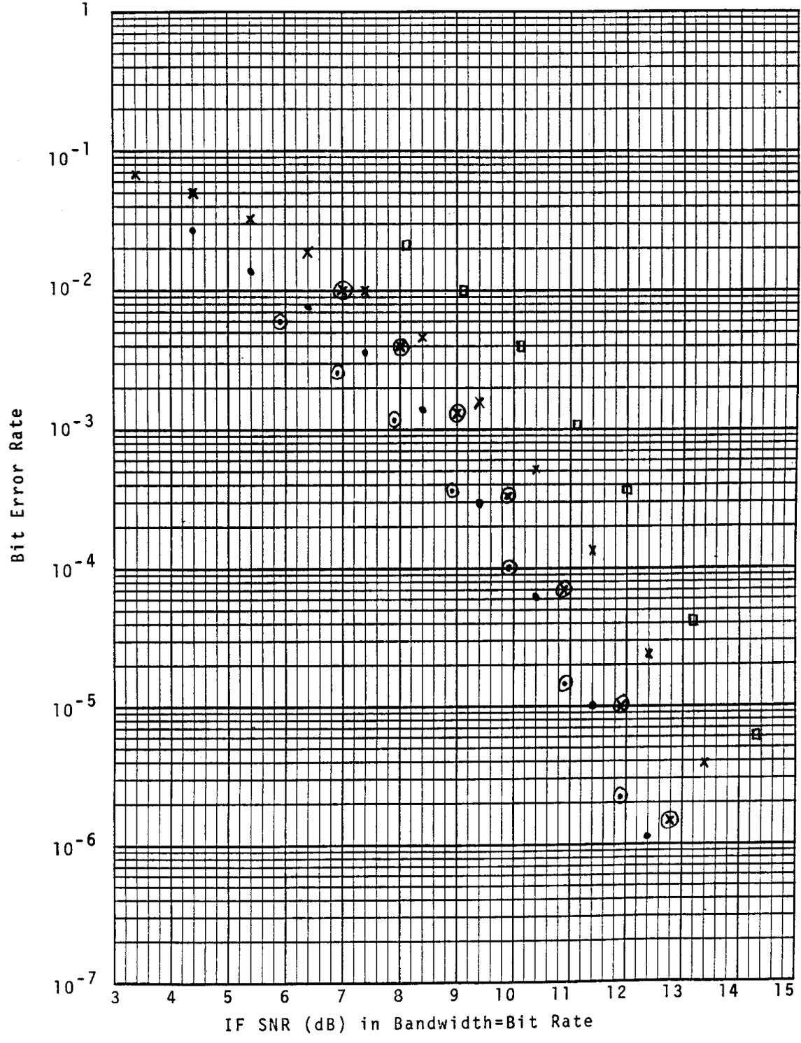
Figure 3. BER versus IF SNR for several PCM formats.
