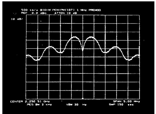
**Figure 2J. BI0-M PCM/PM( $\pm 107^\circ$ )
