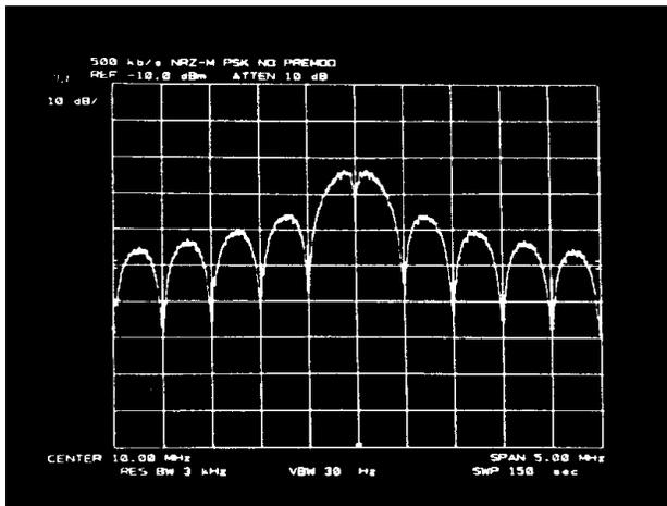
**Figure 2C. NRZ-M PSK No Premodulation Filter.**
