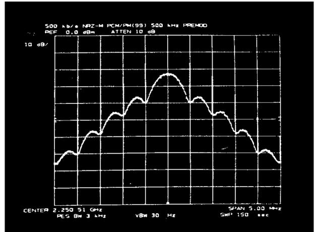
**Figure 2E. NRZ-M PCM/PM( $\pm 99^\circ$ )
