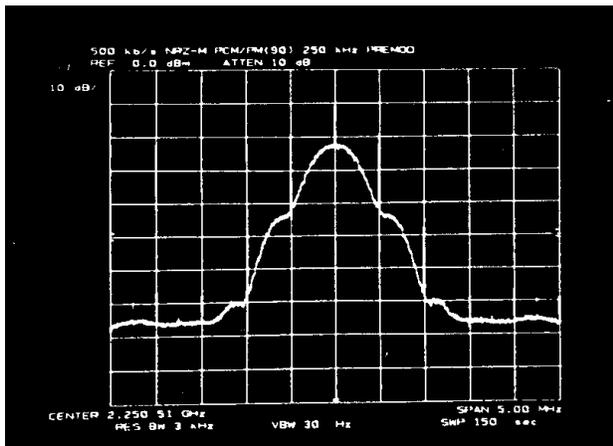
**Figure 2F. NRZ-M PCM/PM( $\pm 90^\circ$ )
