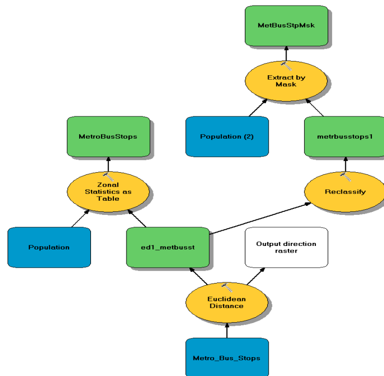
Figure 1: The model process that was used for all of the public transportation datasets used in this project. It includes the Euclidean Distance tool, Zonal Stats as Table, Reclassify, and Extract by Mask
