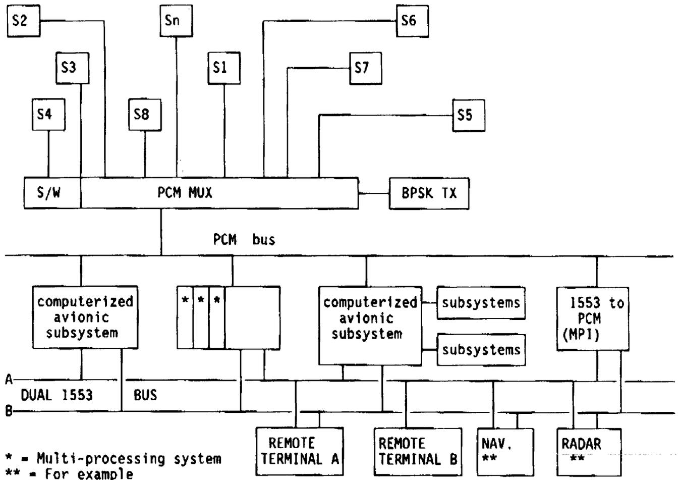
Fig.2: Typical Avionic System Data Acquisition Solution
