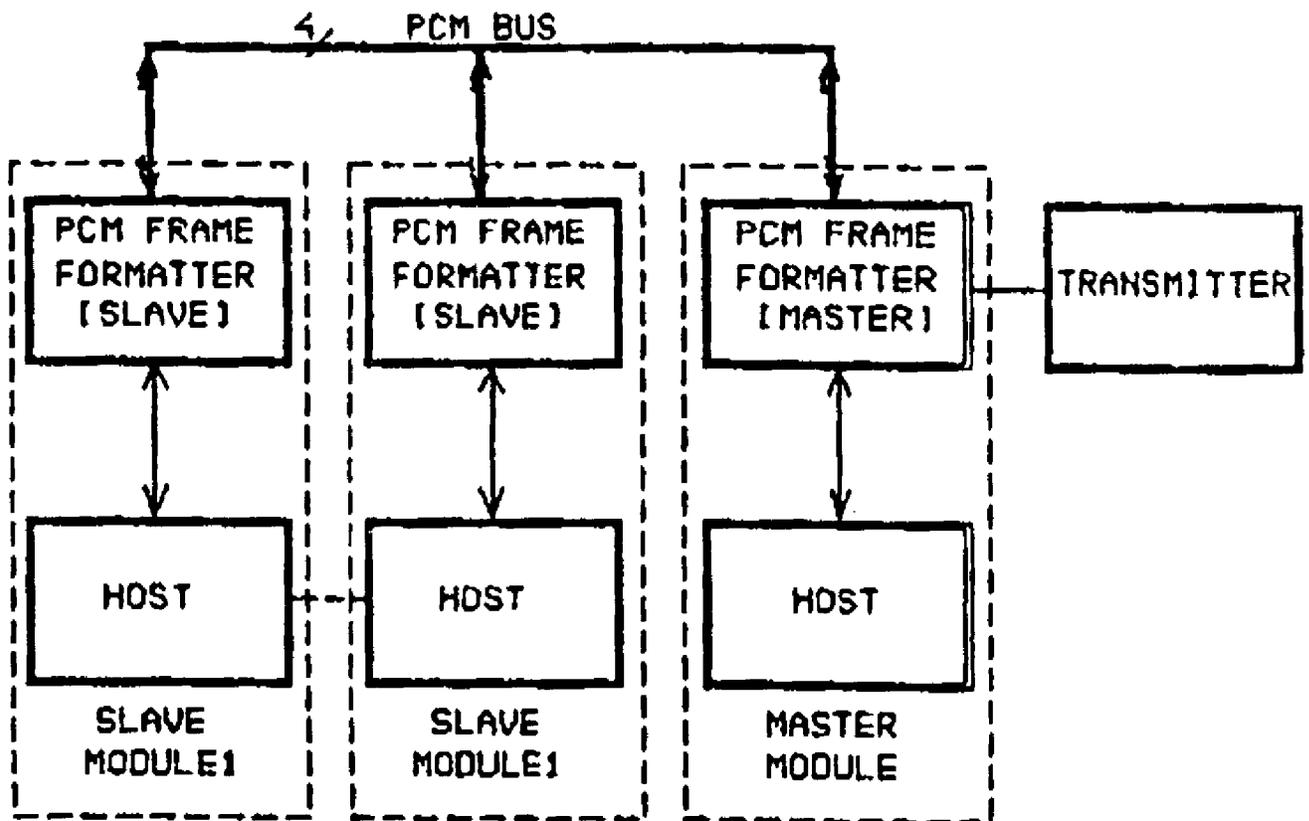
**Fig.3: Multiple Processor Modules Configuration**
