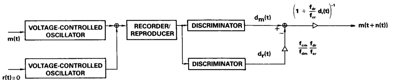
Figure 6. Block Diagram of Tape Speed Compensation Algorithm
