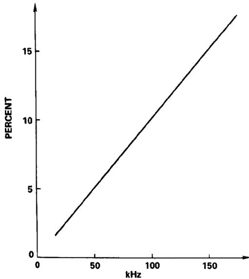
Figure 4. Relative Error Versus Center Frequency for IRIG A Channels
