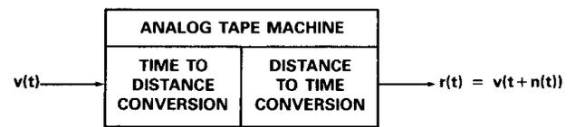
**Figure 2. Independent Variable Conversions Introduce the Time Base Error,  $n(t)$**
