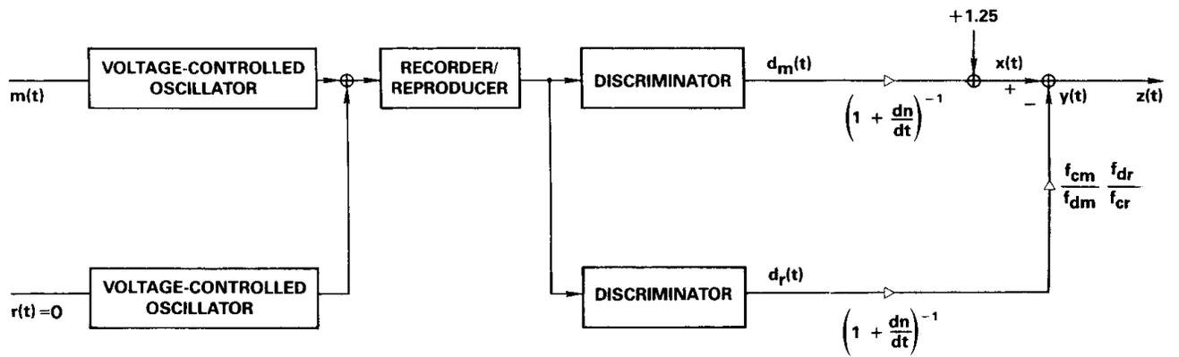
Figure 7. Block Diagram of Empirical Confirmation Experiment
