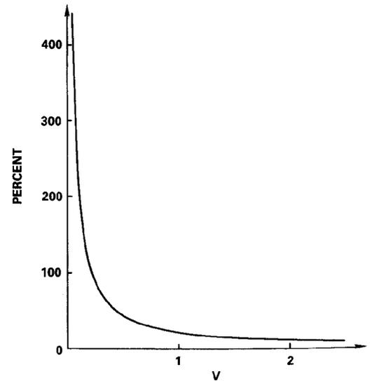
Figure 5. Relative Error Versus Message Amplitude for IRIG Channel 21 A
