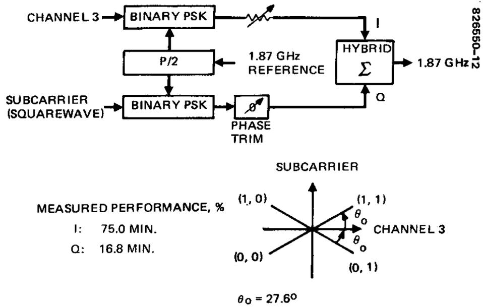
FIGURE 8. RF UNBALANCED QPSK MODULATOR FOR MODE 1
