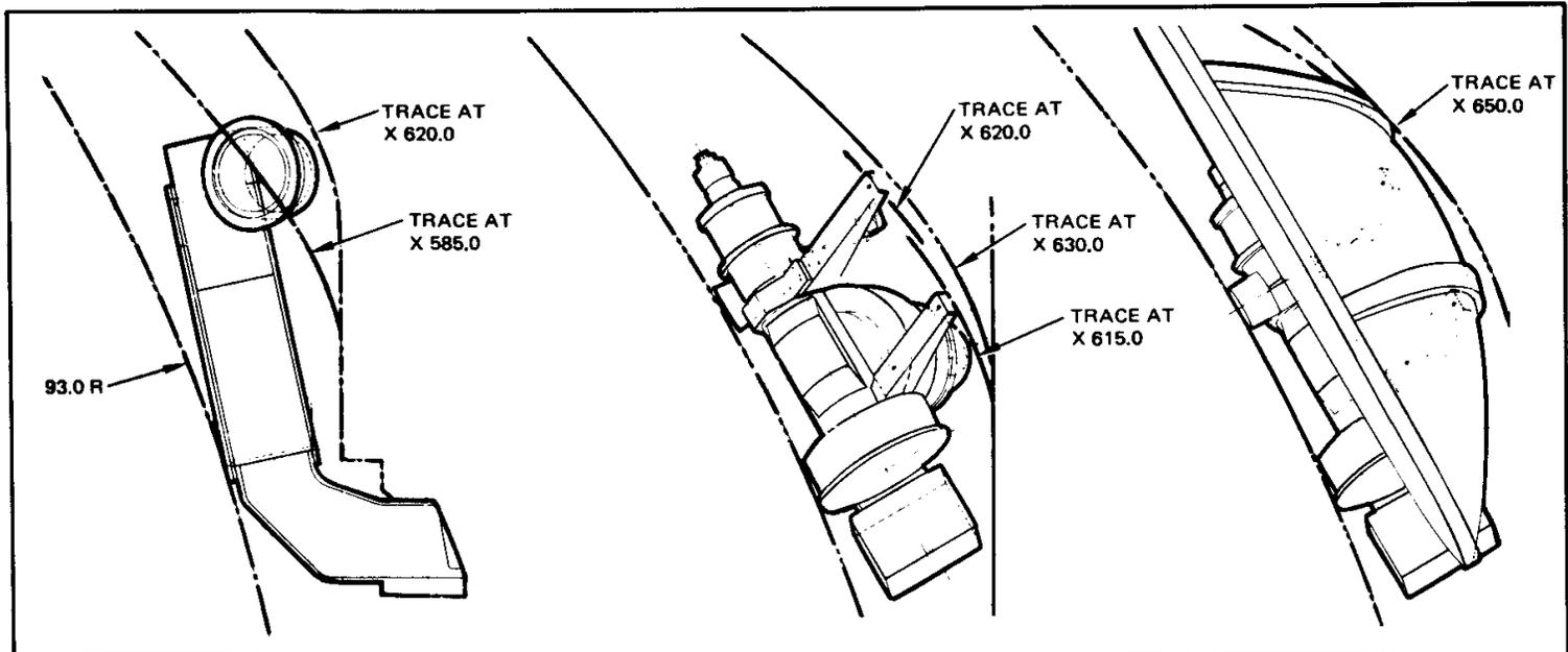
**FIGURE 2. STOWED ANTENNA WITH PAYLOAD BAY DOORS CLOSED**
