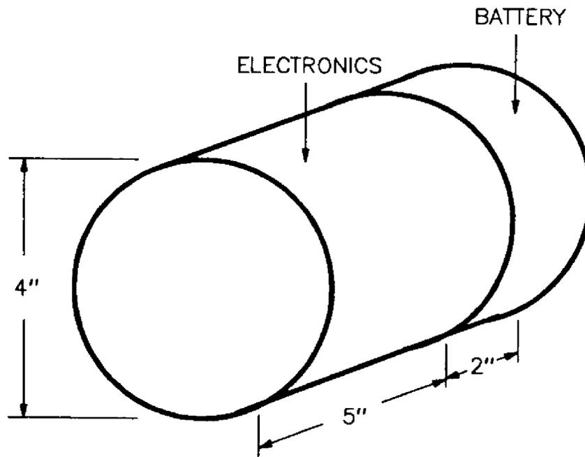
Figure 2. Mechanical Layout
