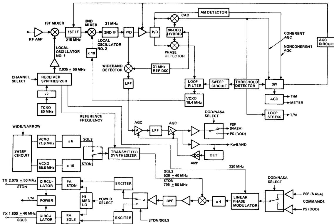
Figure 2. Payload Interrogator Receiver and Transmitter Functional Block Diagram
