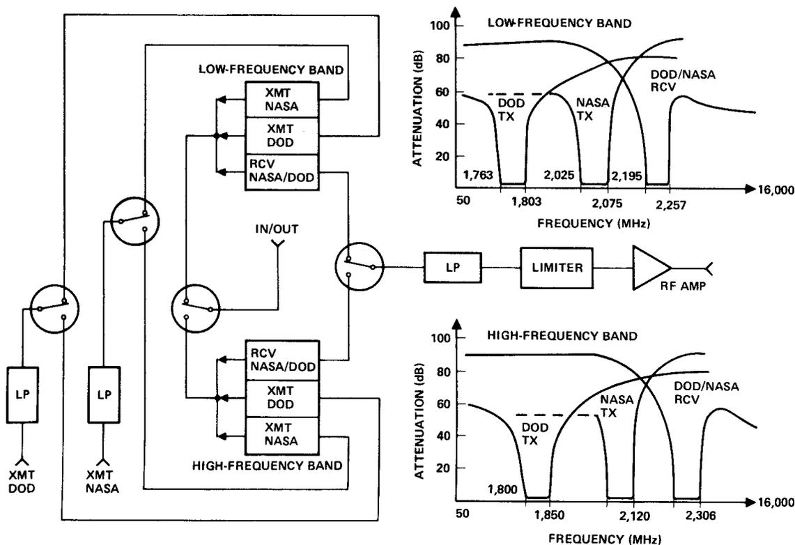
Figure 1. Dual Triplexer Block Diagram and Its Frequency Response
