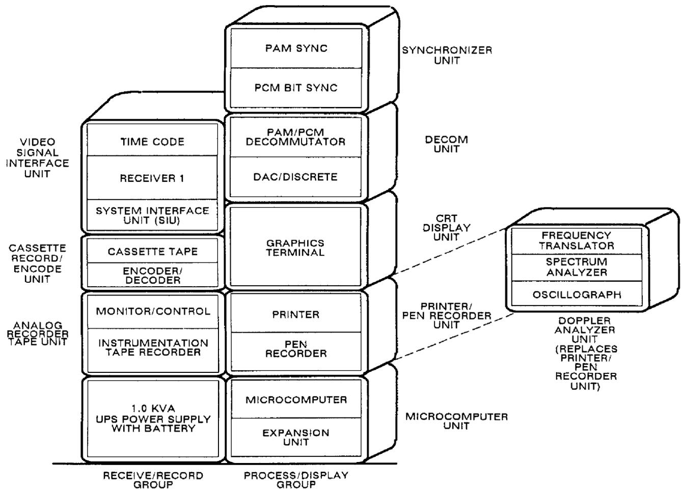
Figure 2 AERO Physical Layout - Outline of Equipment During Operation
