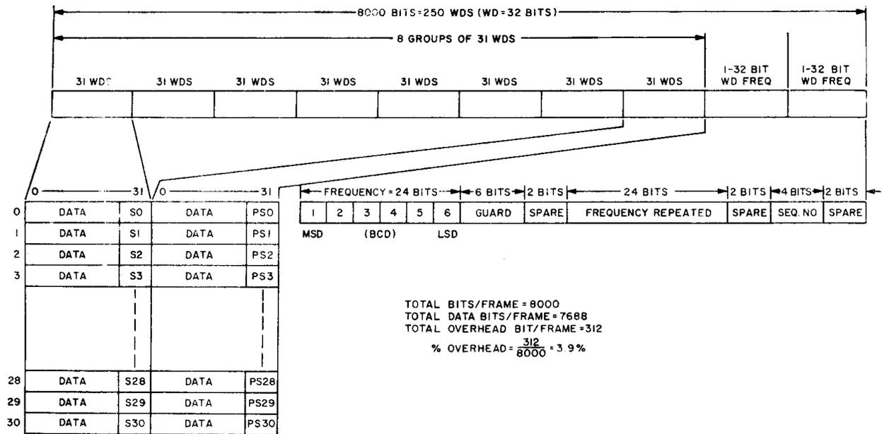
S0 THRU S30 IS ONE OF FOUR 31 BIT PN SEQUENCES USED AS A DISTRIBUTED WORD BOUNDARY SYNC PATTERN AND FOR PORT IDENTIFICATION
