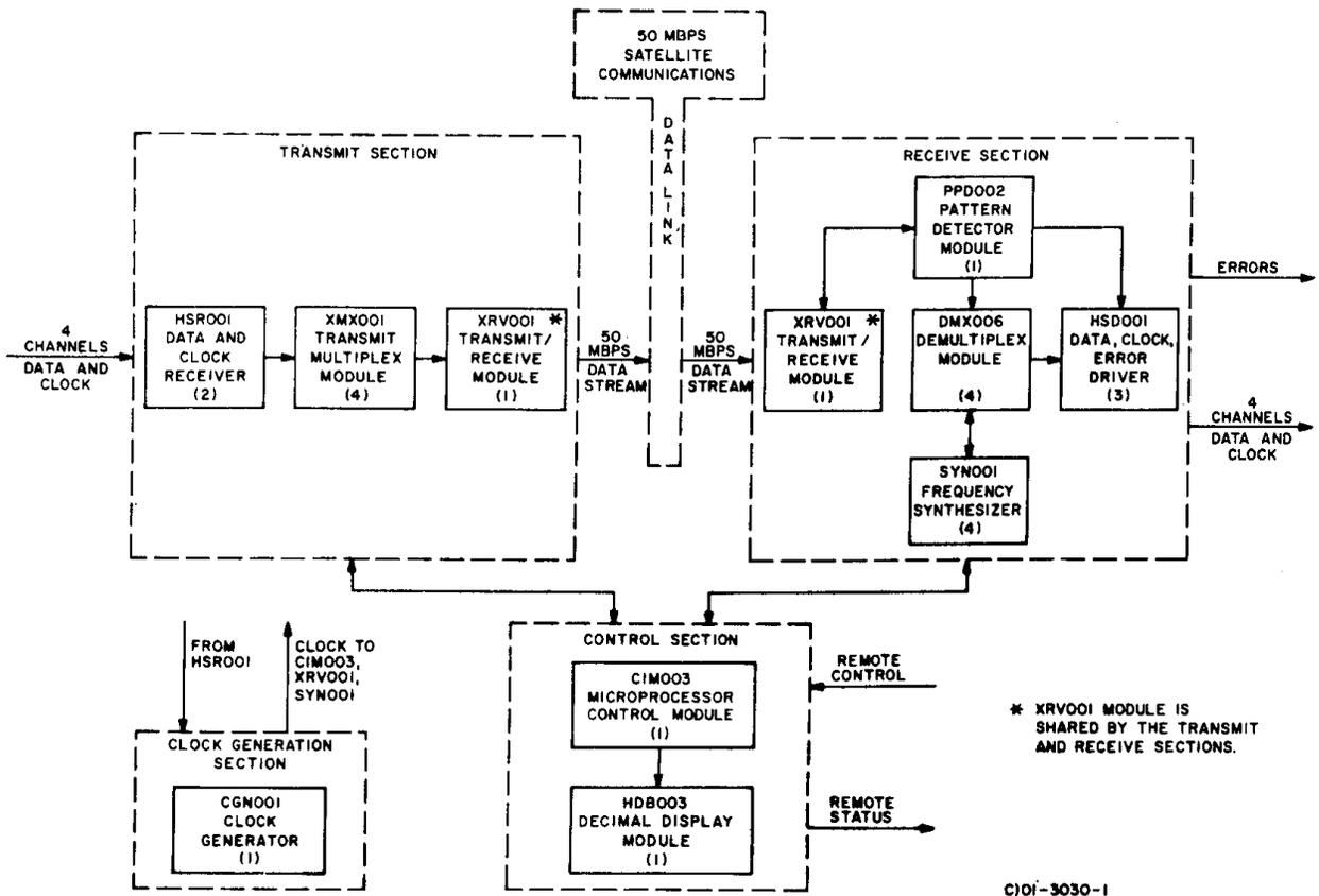
Figure 2 - Model 781 Simplified Block Diagram
