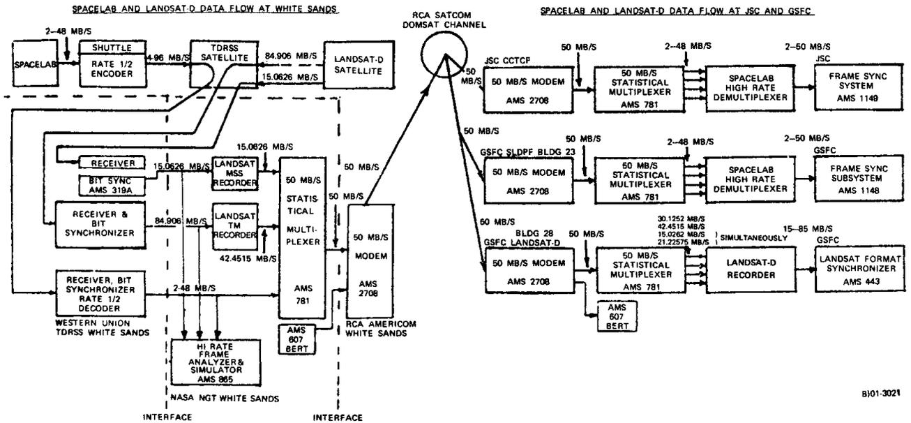
Figure 4 - Spacelab/Landsat Data Communications Network
