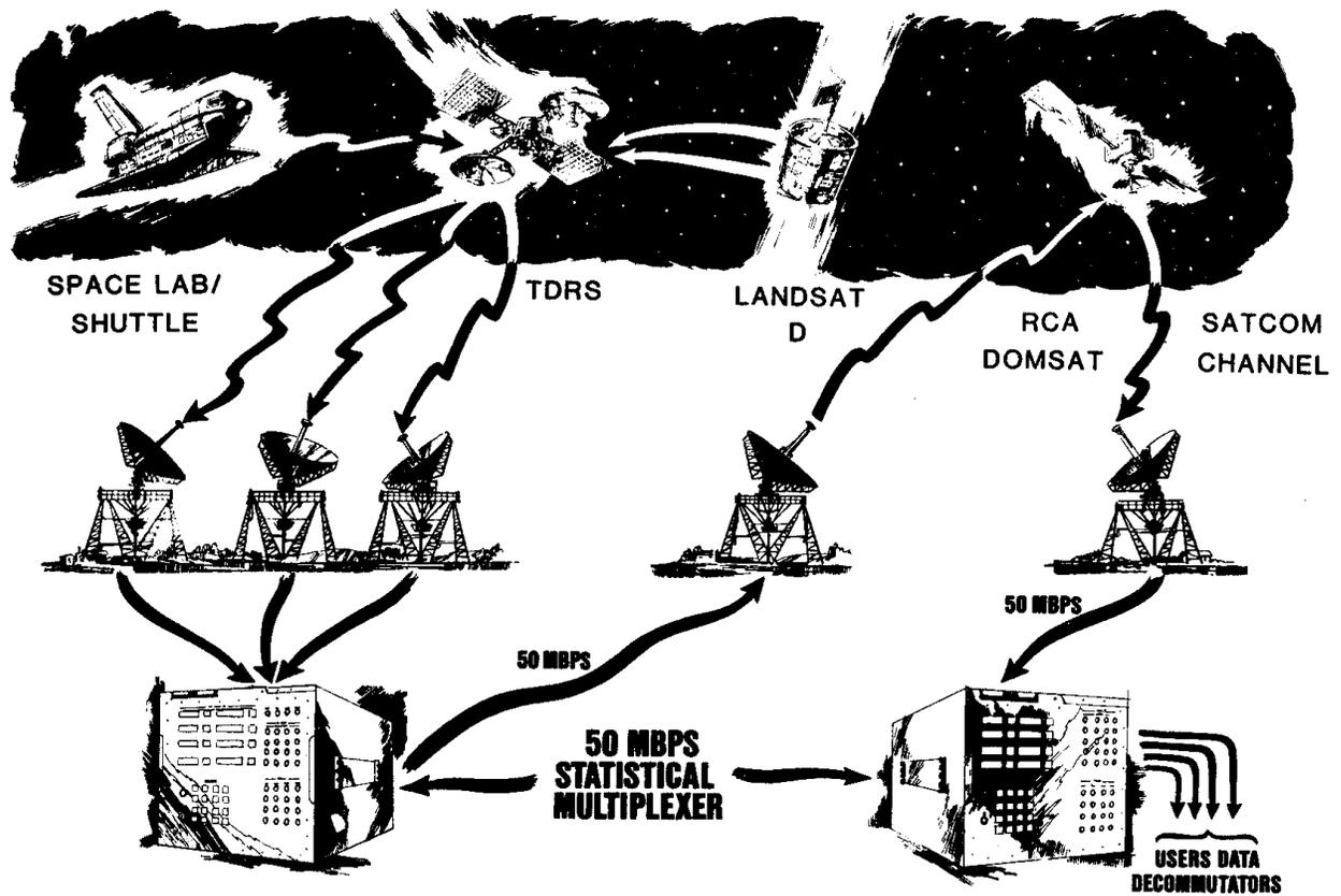
Figure 3 - Spacelab/Landsat Data Flow
